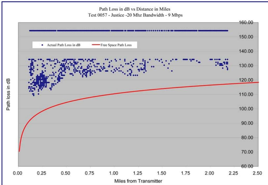
Graph 4.29 – Justice Center - 20 MHz / 9 Mbps – Path Loss versus Distance
