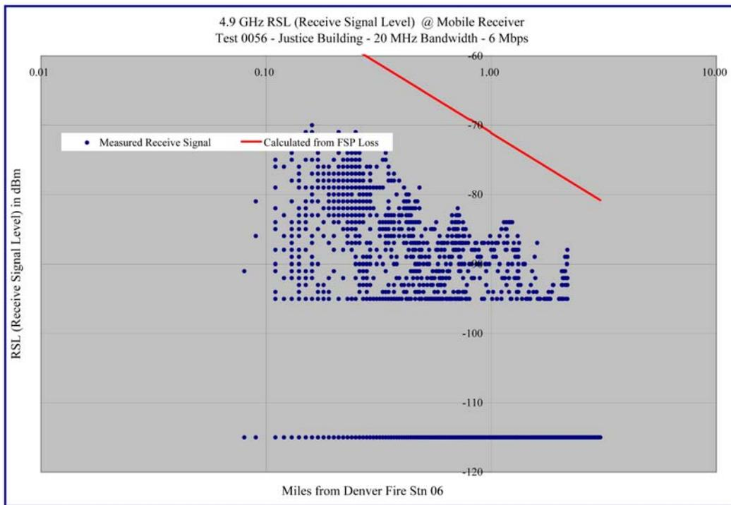
Graph 4.19 Justice Center – Receive Signal Level versus Distance – 20 MHz / 6 Mbps – Log-Log Format
