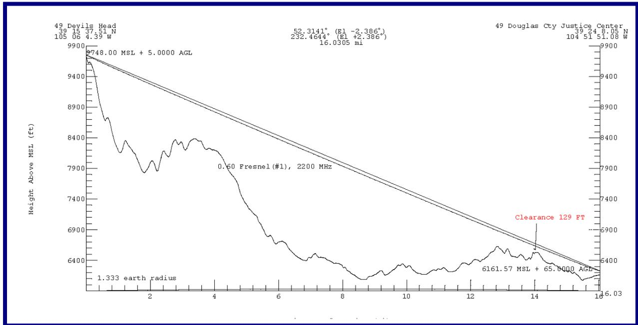
Figure 3.1 Microwave Path Profile from Devil's Head to Douglas County Justice Center
