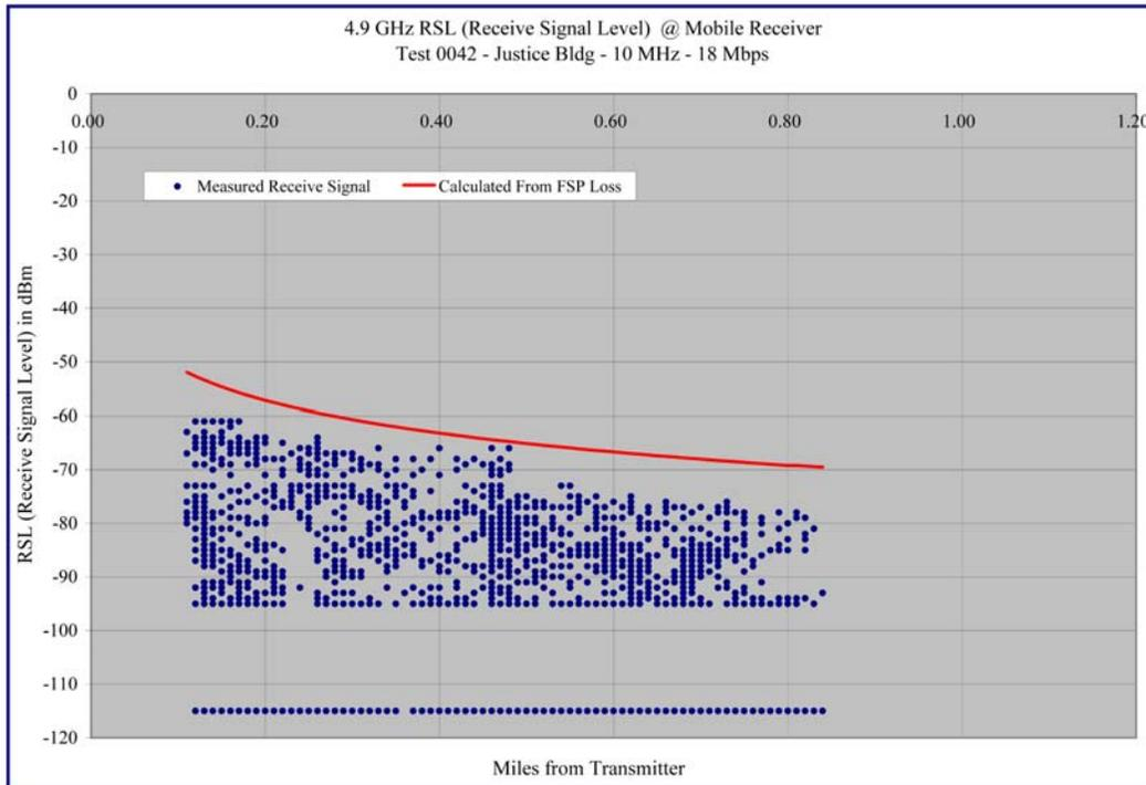
**Graph 4.41 – Justice Center – 10 MHz / 18 Mbps - Receive Signal Strength versus Distance**
