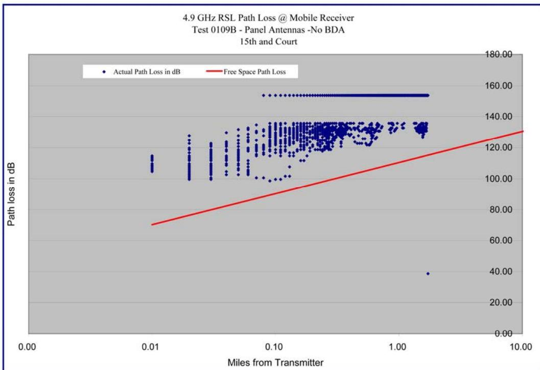
**Graph 6.40 Path Loss versus Distance – 15<sup>th</sup> and Court Place – Log-Log Format**
