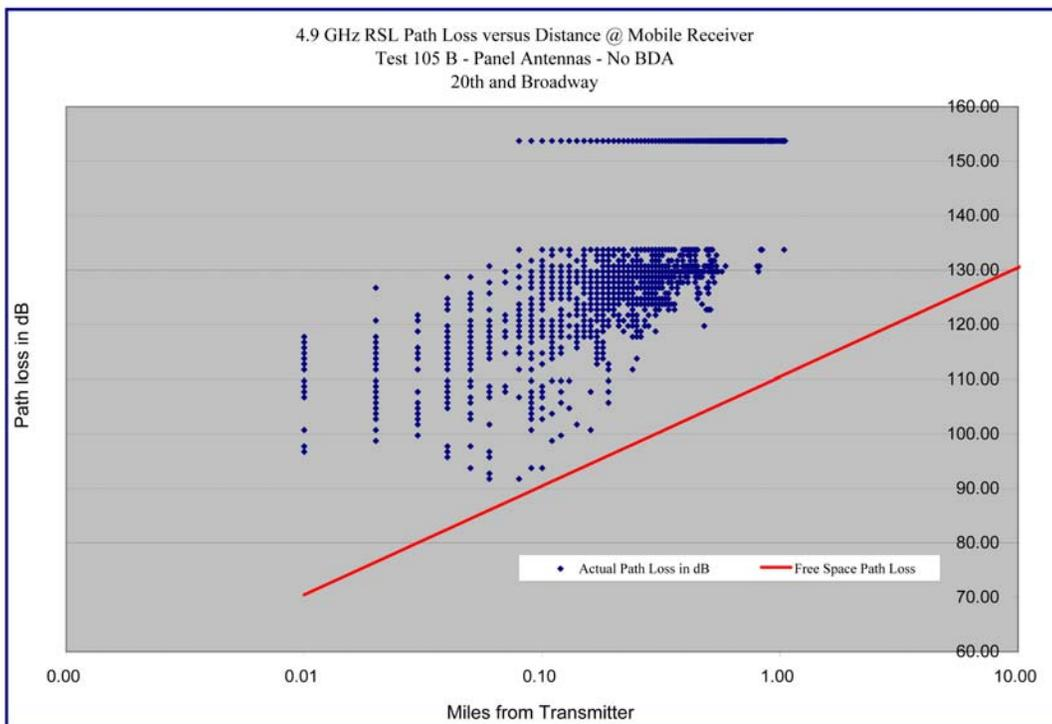
**Graph 6.8 – Path Loss versus Distance – Test 105B – Panel Antennas no BDA – Log-Log Format**
