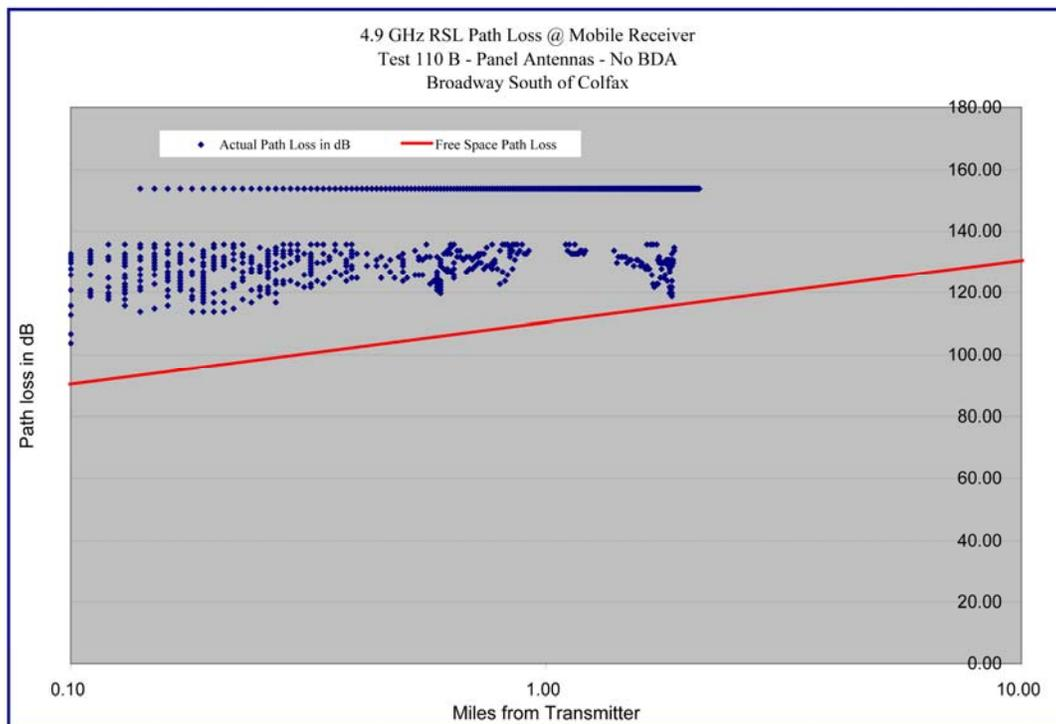
**Graph 6.48 Path Loss versus Distance – Broadway South of Colfax – Log-Log Format**
