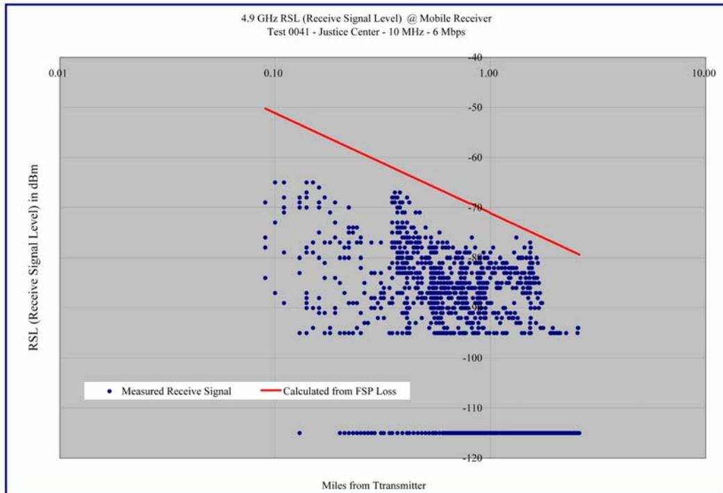
**Graph 4.11 – Justice Center -10 MHz/ 6 Mbps - Receive Signal versus Distance- Log-Log Format**
