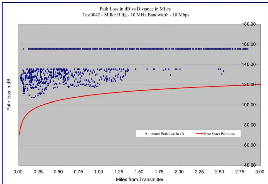
**Graph 4.46 – Miller Building -10 MHz / 18 Mbps - Path Loss versus Distance**
