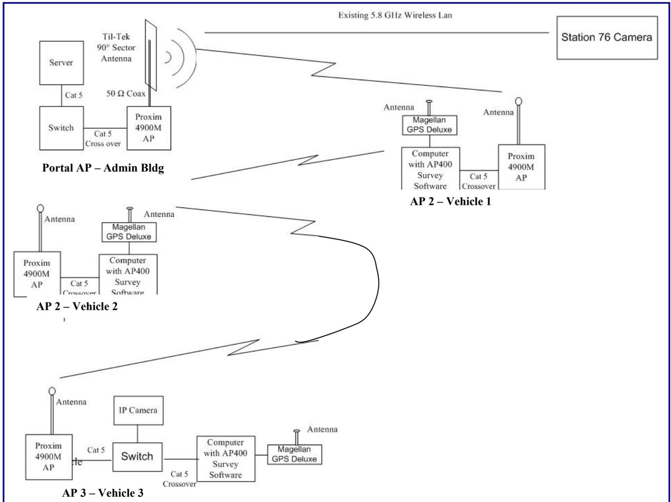
Figure 8.2 – Ad Hoc Testing Configuration
