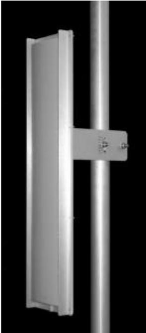
The TA-4904-14-90 is a vertically polarized 90 degree sectoral antenna. The antenna consists of a printed dipole array enclosed in an aluminum base with a UV stabilized radome for superior weatherability. The antenna is at DC ground to aid in lightning protection.
