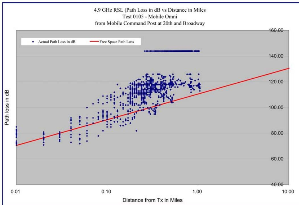
**Graph 6.4 – Path Loss versus Distance – Test 105 Omni with BDA – Log-Log Format**
