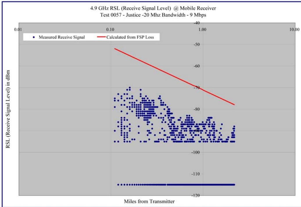
**Graph 4.27 – Justice Center - 20 MHz / 9 Mbps – Receive Signal Strength versus Distance – Log-Log Format**
