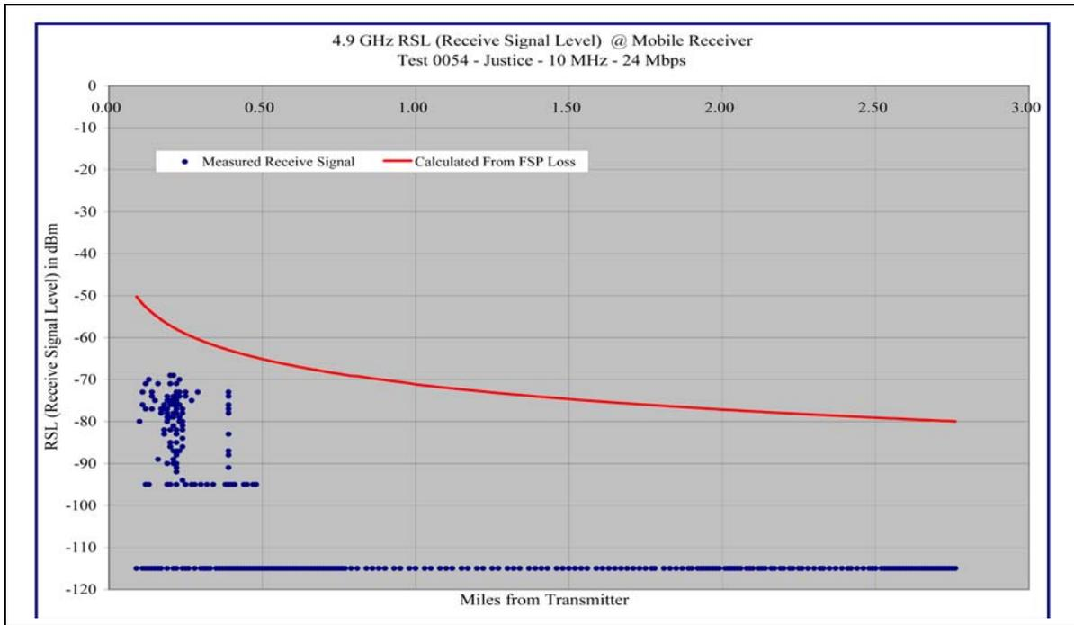
Graph 4.53 Justice Center – 10 MHz / 24 Mbps – Receive Signal Strength versus Distance
