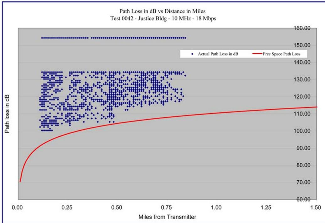
**Graph 4.45 – Justice Center -10 MHz / 18 Mbps - Path Loss versus Distance**
