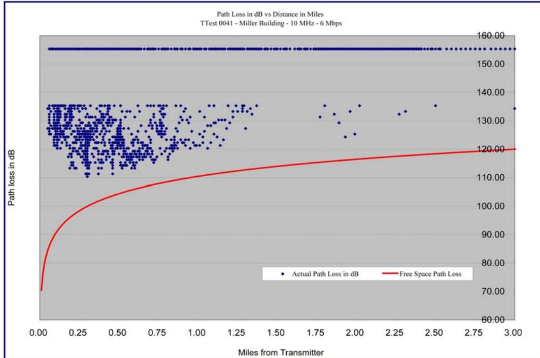
**Graph 4.15– Miller Building –10 MHz / 6 Mbps - Path Loss versus Distance**
