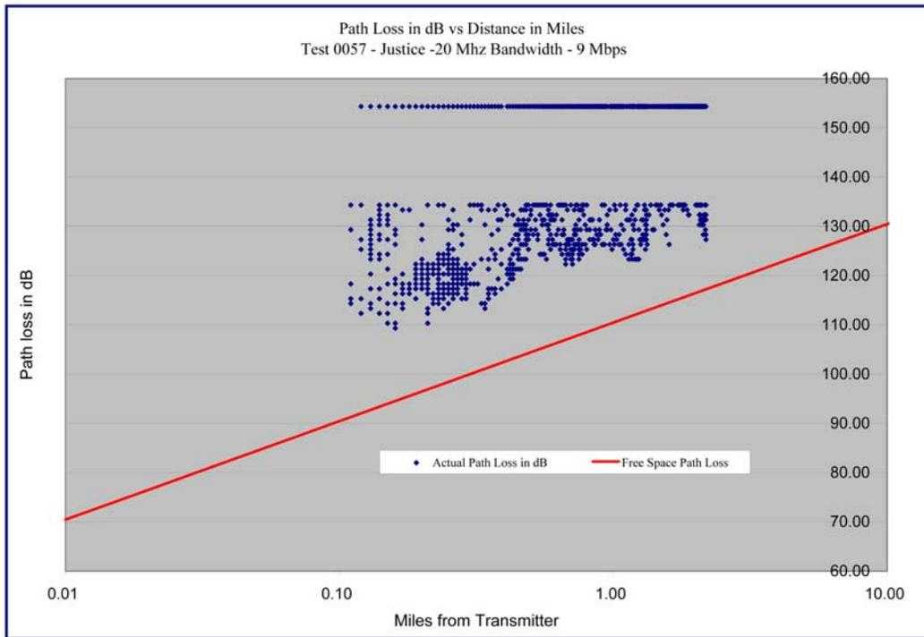
**Graph 4.31 – Justice Center - 20 MHz / 9 Mbps – Path Loss versus Distance – Log-Log Format**
