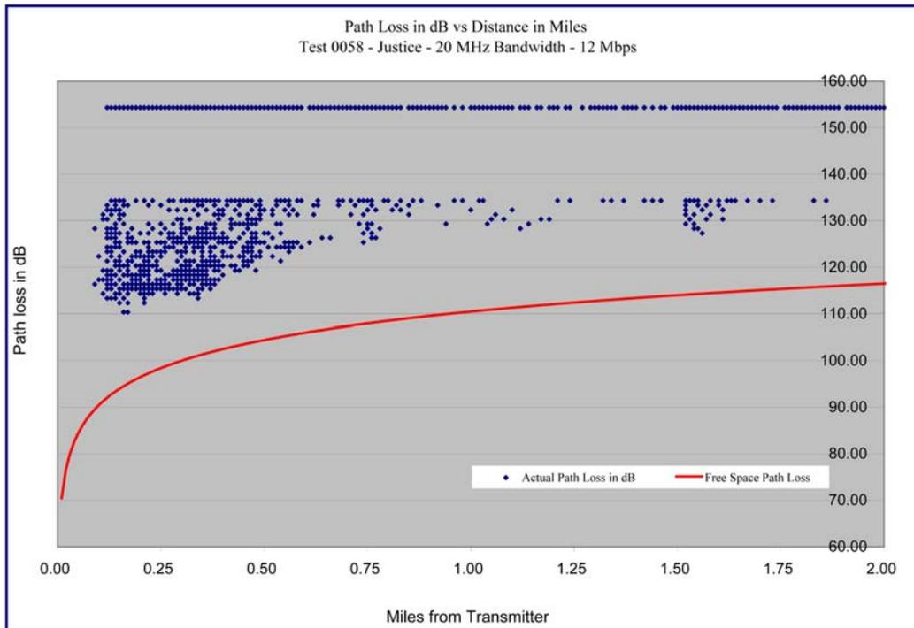
**Graph 4.37 – Justice Center – 20 MHz / 12 Mbps - Path Loss versus Distance**
