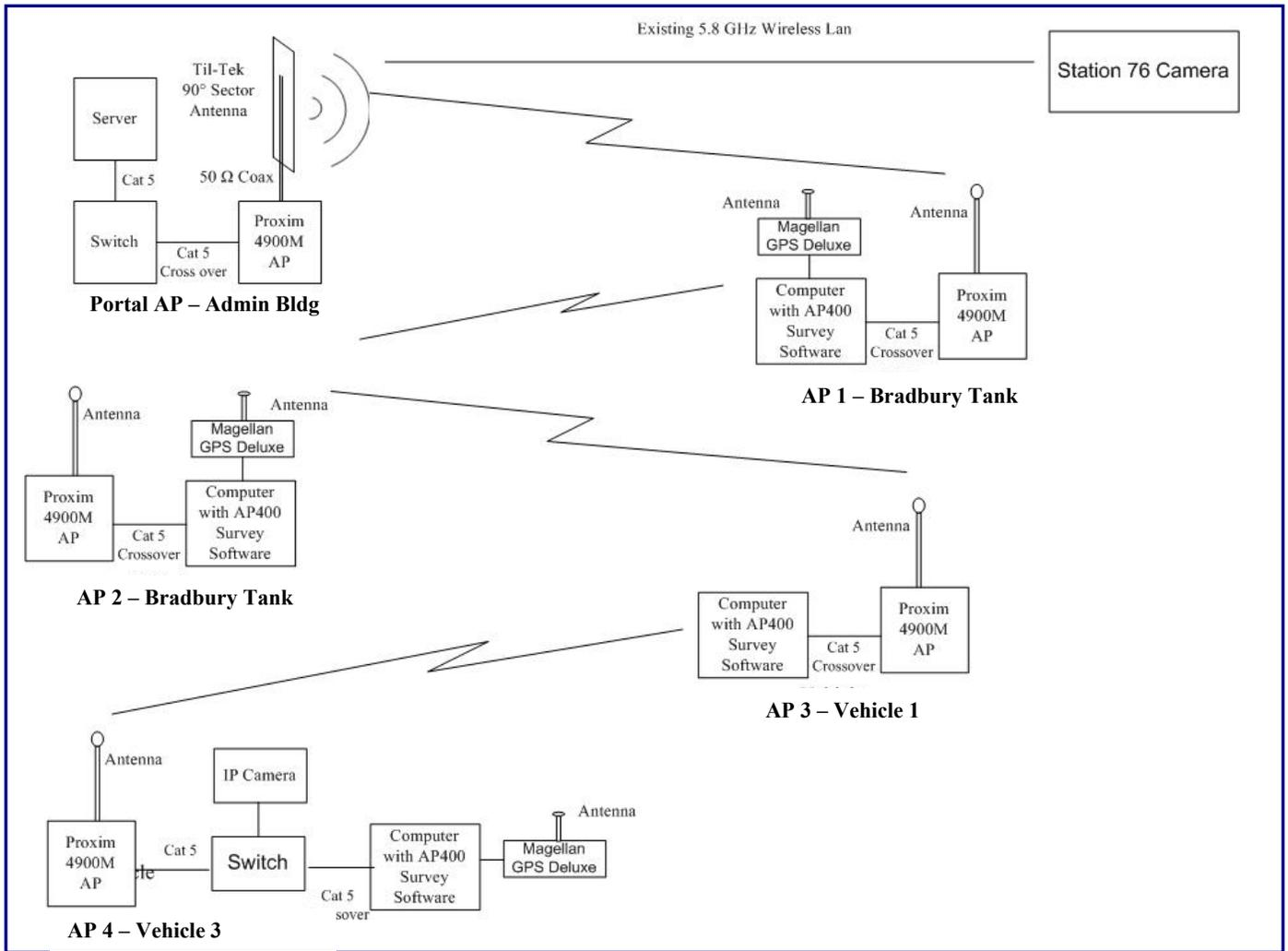
Figure 8.3 – Ad Hoc Testing Configuration
