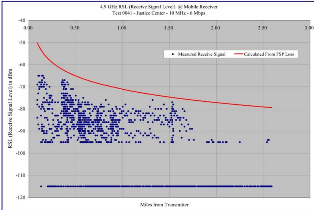
**Graph 4.9 – Justice Center - 10 MHz/ 6 Mbps – Receive Signal versus Distance**
