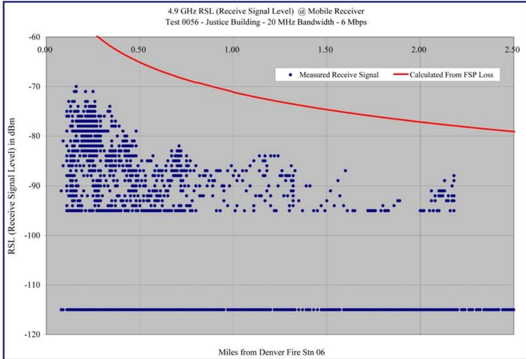
**Graph 4.17 – Justice Center – 20 MHz / 6 Mbps - Receive Signal versus Distance**
