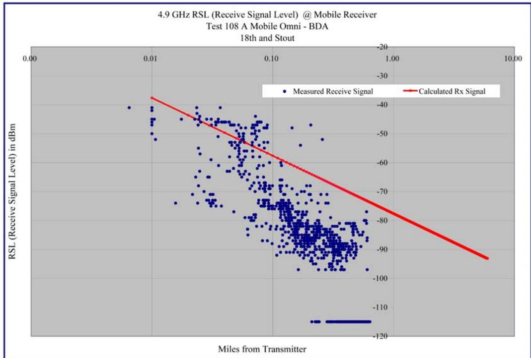
Graph 6.26 – Receive Signal Level versus Distance – 18<sup>th</sup> and Stout – Log-Log Format
