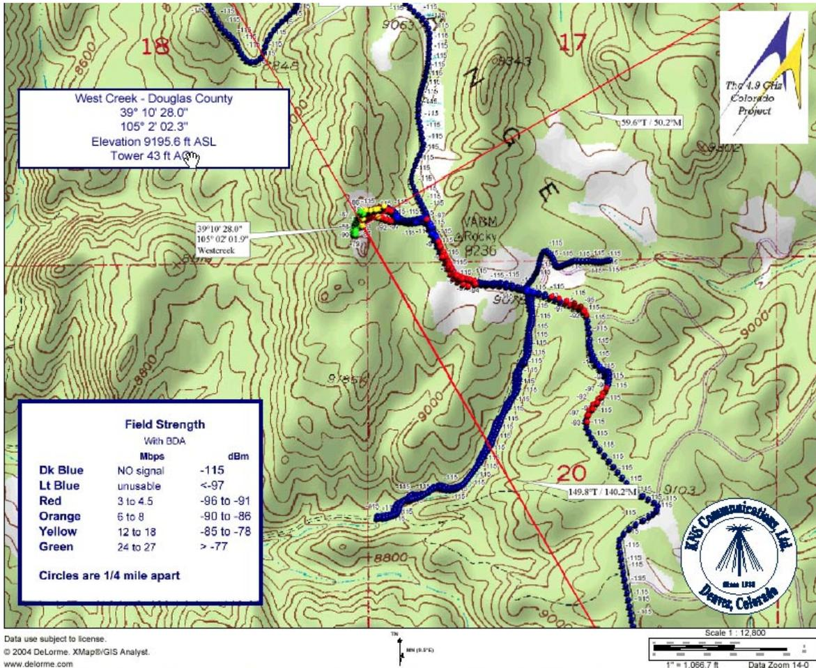
Figure 19 - West Creek Coverage (EIRP = 31 dBm)
