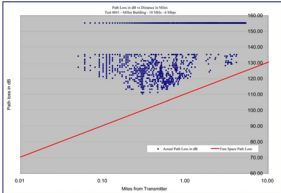
**Graph 4.16– Miller Building – 10 MHz / 6 Mbps - Path Loss versus Distance – Log-Log Format**
