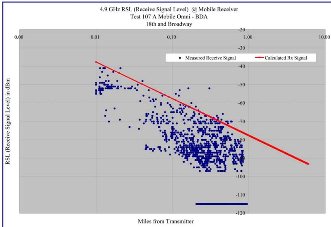
**Graph 6.18 – Receive Signal Level versus Distance – Test 107 - 18<sup>th</sup> and Broadway – Log-Log Format**
