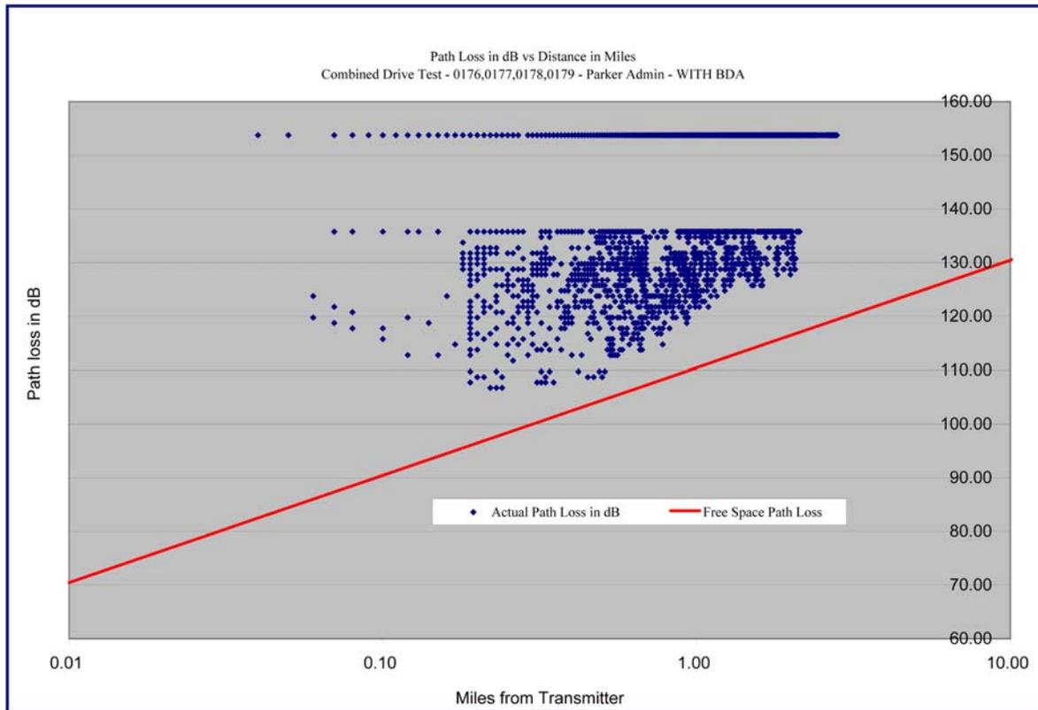
**Graph 2.4 - Measured Free Space Path Loss Versus Distance – Log-Log Format**
