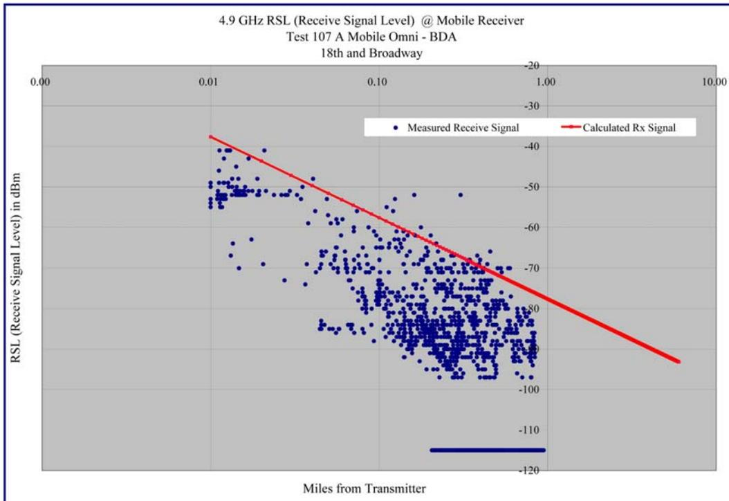
Graph 6.20 – Path Loss versus Distance – Test 107 - 18<sup>th</sup> and Broadway – Log-Log Format
