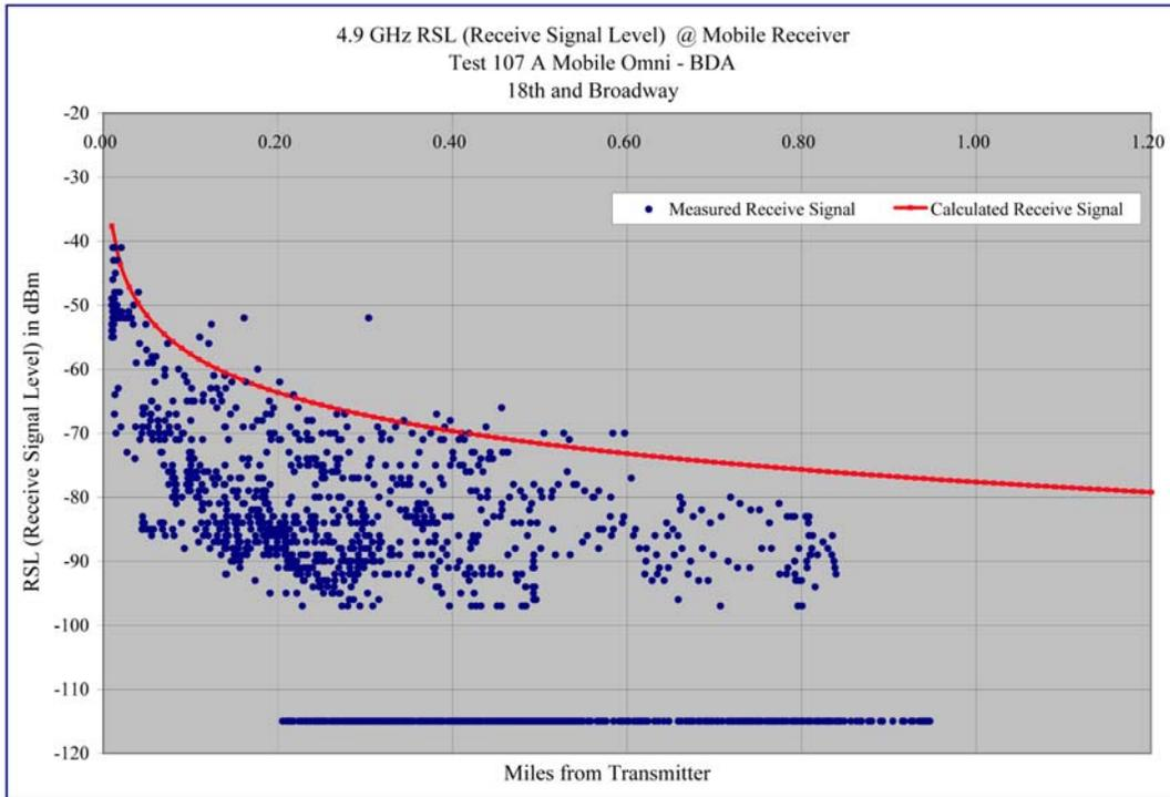
**Graph 6.17 – Receive Signal Level versus Distance – Test 107 - 18<sup>th</sup> and Broadway**
