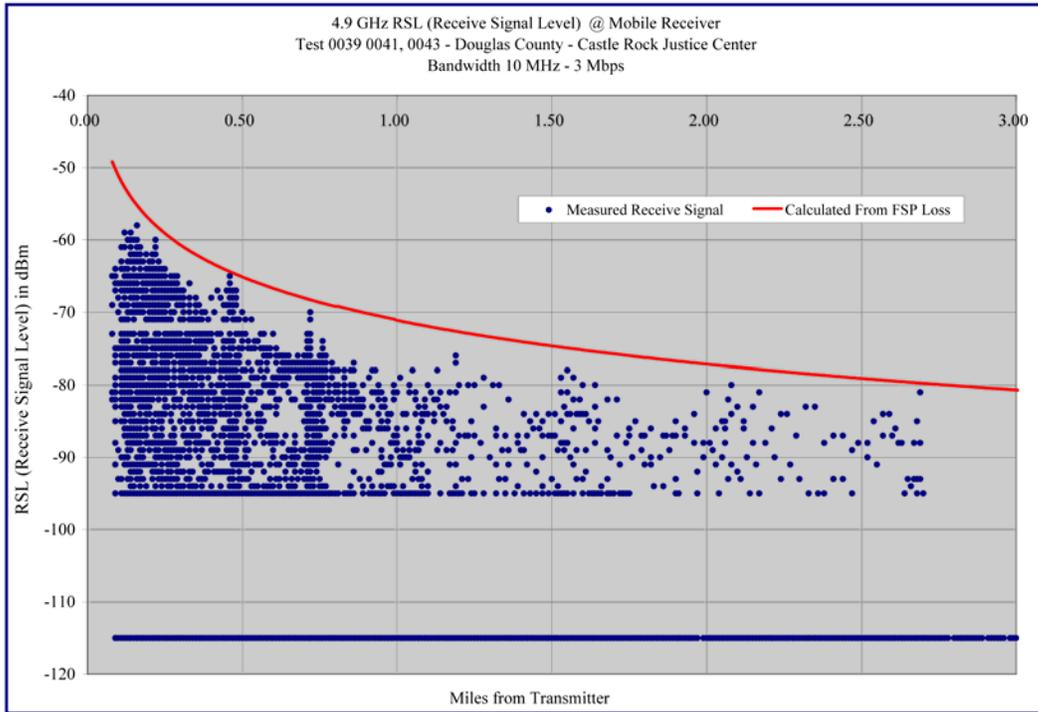
**Graph 4.1 - Justice Center – 10 MHz / 3 Mbps -Receive Signal Level versus Distance**
