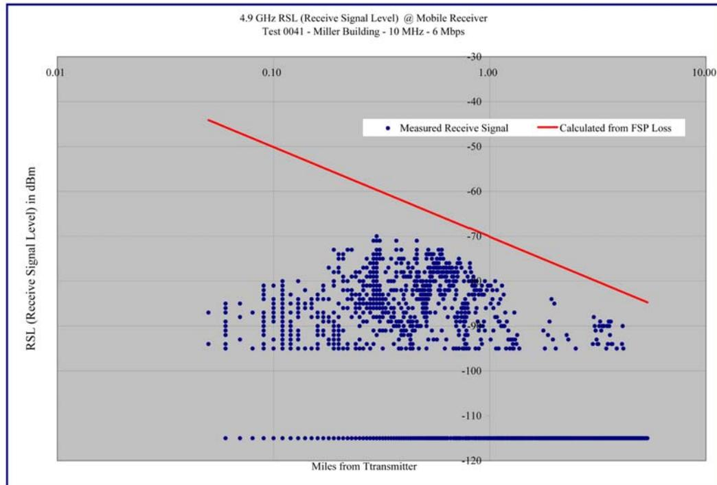
**Graph 4.12 – Miller Building – 10 MHz / 6 Mbps - Receive Signal Level versus Distance — Log-Log Format**
