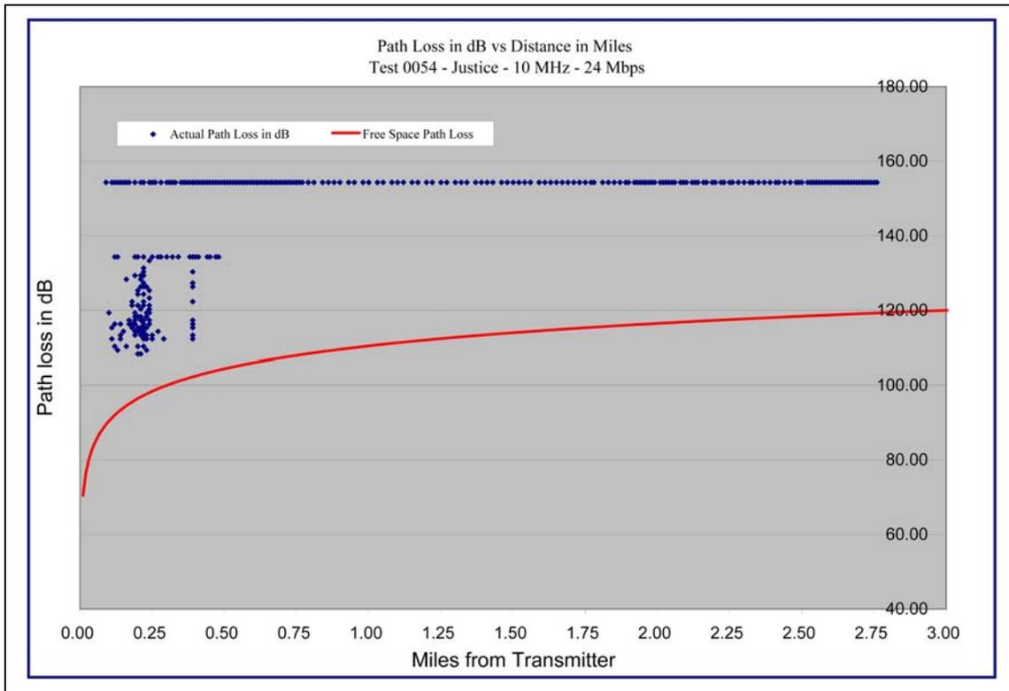
**Graph 4.55 – Justice Center - 10 MHz / 24 Mbps – Path Loss versus Distance**
