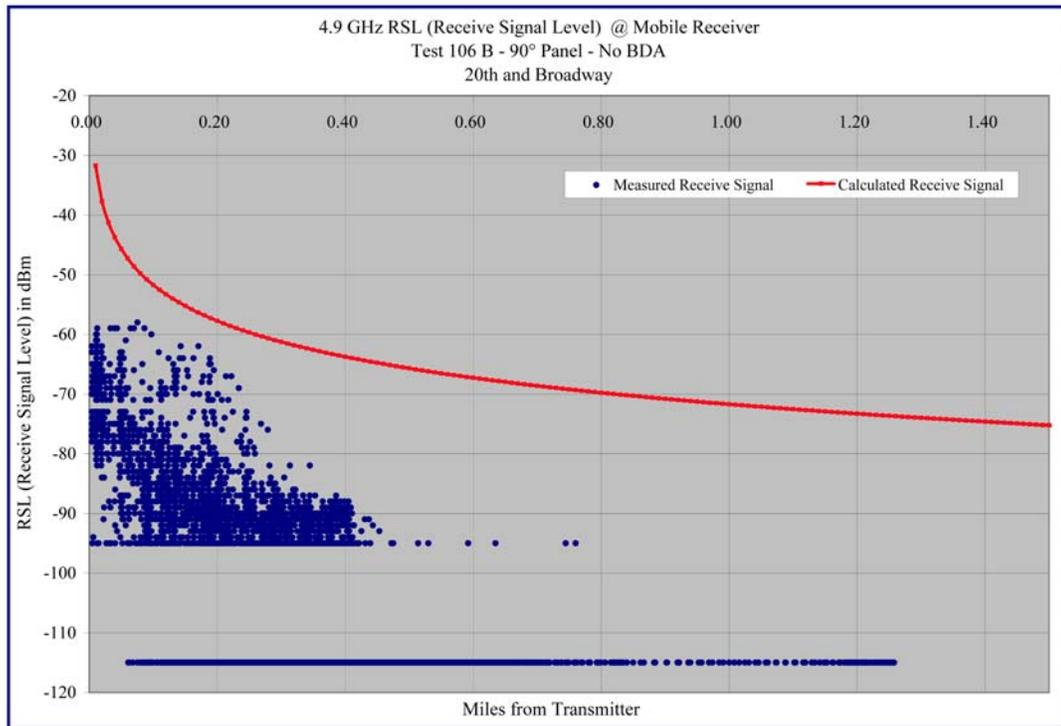
**Graph 6.13 – Receive Signal Level versus Distance – 20<sup>th</sup> and Broadway Test B**
