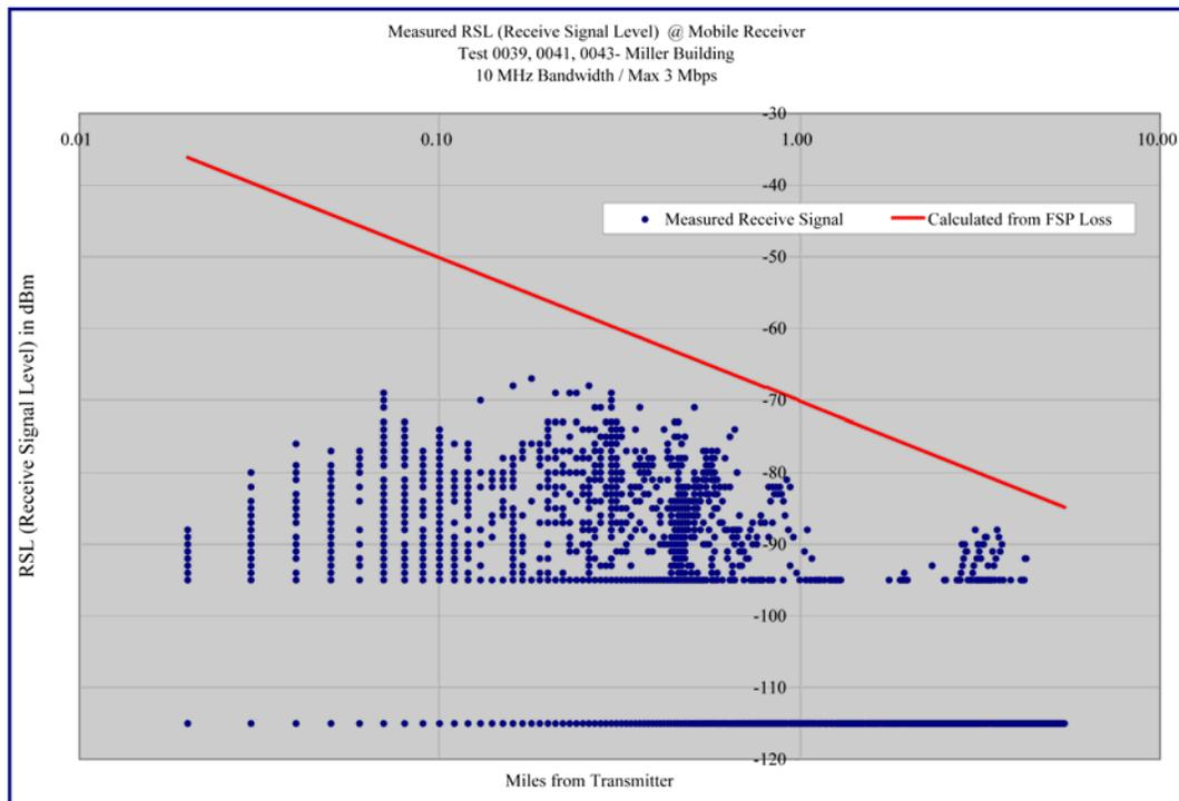
**Graph 4.4 – Miller Building – 10 MHz / 3 Mbps - Receive Signal Level Versus Distance-Log-Log**
