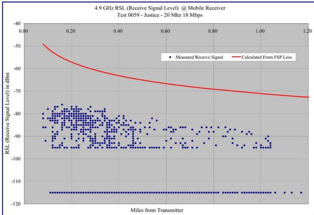
**Graph 4.49 – Justice Center – 20 MHz / 18 Mbps - Receive Signal Strength versus Distance**
