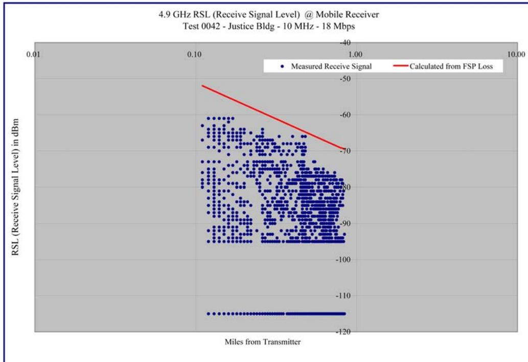
**Graph 4.43 – Justice Center -10 MHz / 18 Mbps - Receive Signal Strength versus Distance- Log-Log Format**
