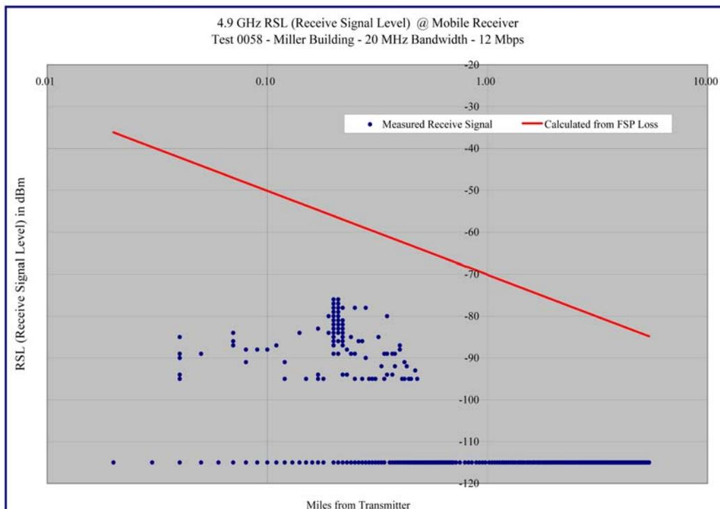
**Graph 4.36 – Miller Building - 20 MHz / 12 Mbps - Receive Signal Strength versus Distance- Log-Log Format**
