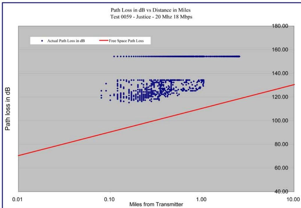
Graph 4.52 – Justice Center – 20 MHz / 18 Mbps - Path Loss versus Distance – Log-Log Format
