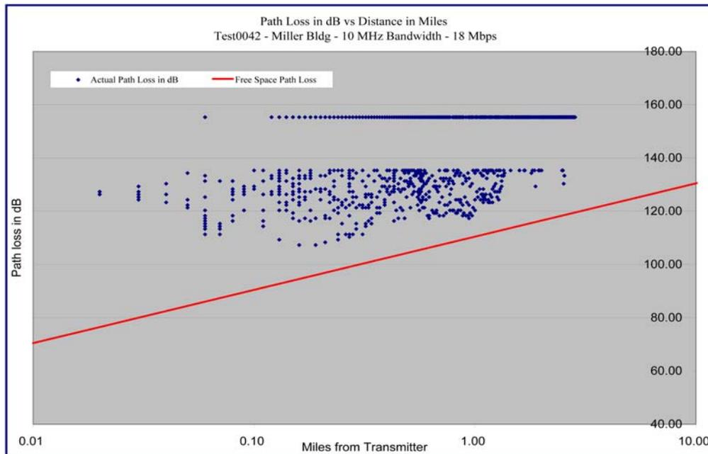
**Graph 4.48 – Miller Building - 10 MHz / 18 Mbps - Path Loss versus Distance – Log-Log Format**
