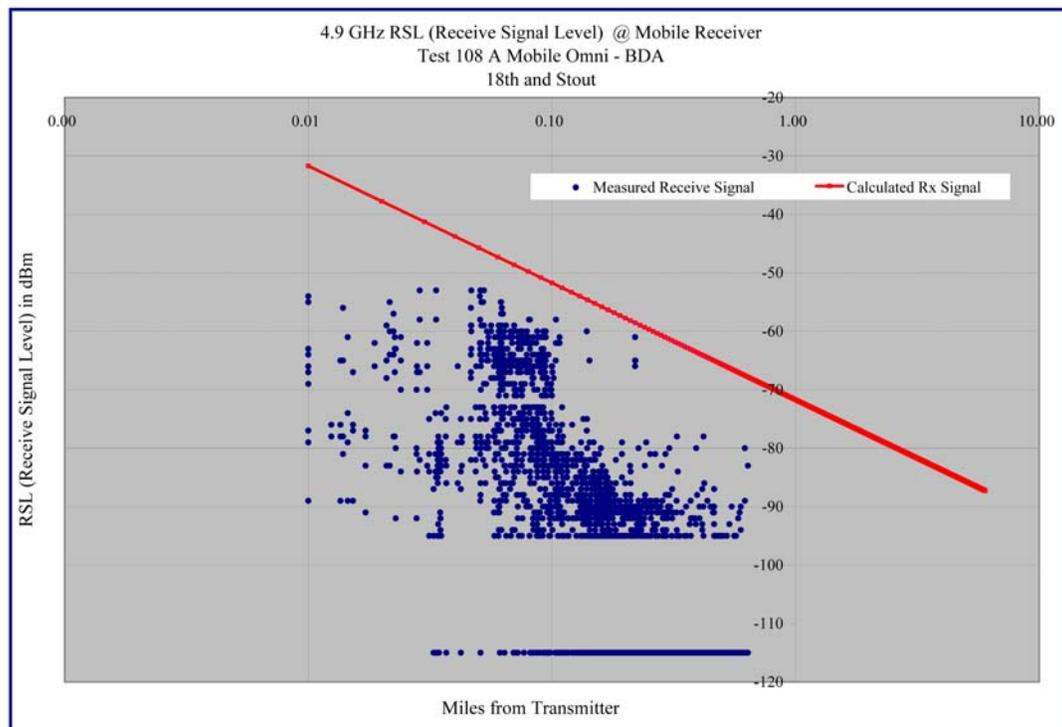
Graph 6.30– Receive Signal Level versus Distance – 18<sup>th</sup> and Stout – Log-Log Format
