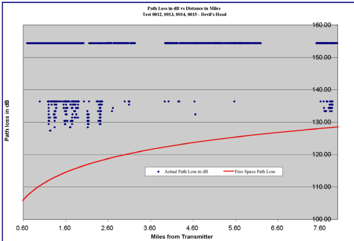
**Graph 3.3 - Measured Path Loss versus Distance – Devil's Head**
