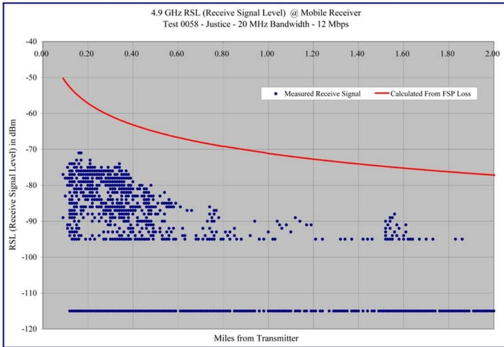
**Graph 4.33 – Justice Center – 20 MHz / 12 Mbps - Receive Signal Strength versus Distance**
