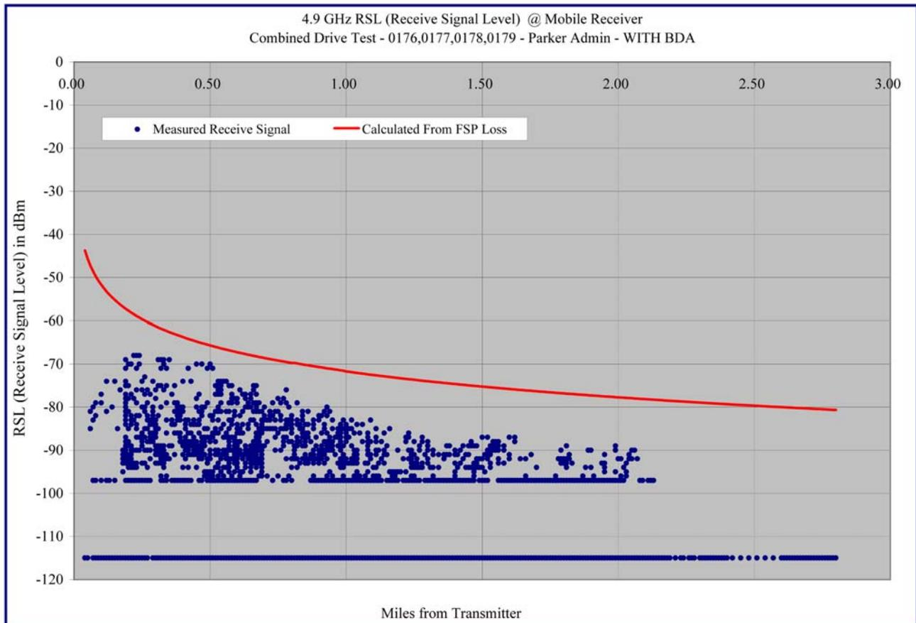
**Graph 2.1 – Measured Receive Signal Level versus Distance**
