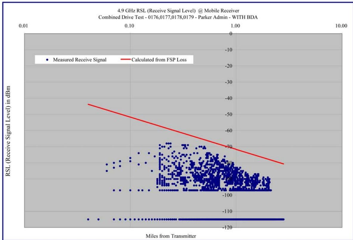
**Graph 2.2 - Measured Receive Signal Level versus Distance – Log-Log Format**
