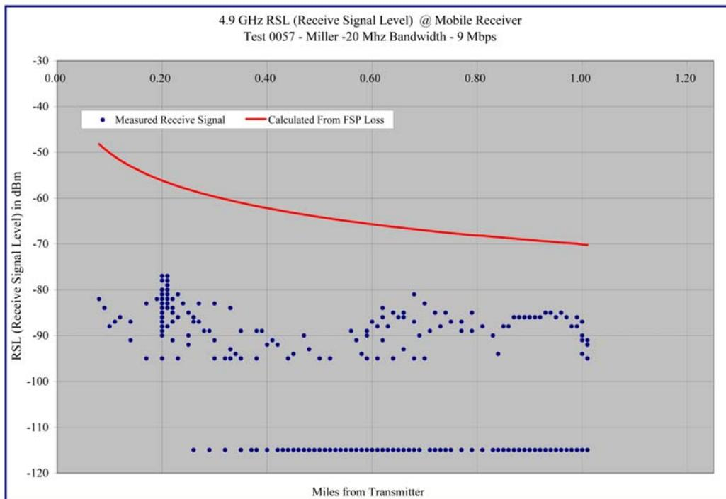
**Graph 4.26 – Miller Building - 20 MHz / 9 Mbps – Receive Signal Strength versus Distance**
