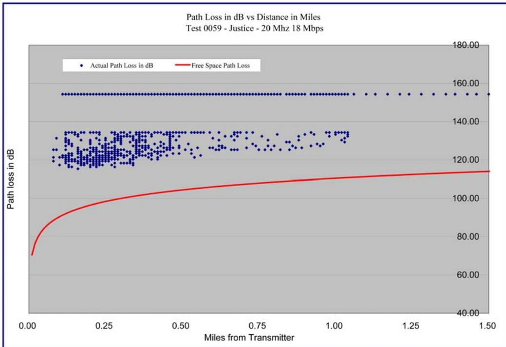
Graph 4.51 – Justice Center – 20 MHz / 18 Mbps - Path Loss versus Distance
