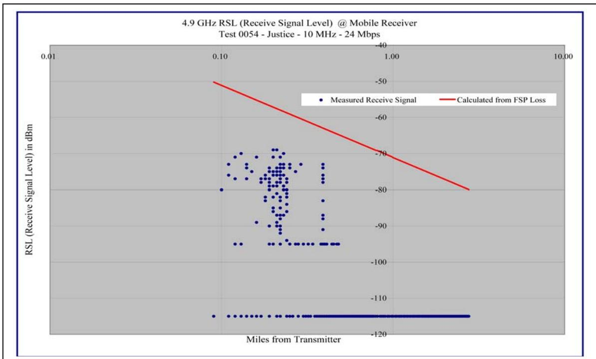
Graph 4.54 Justice Center – 10 MHz / 24 Mbps – Receive Signal Strength versus Distance – Log-Log Format
