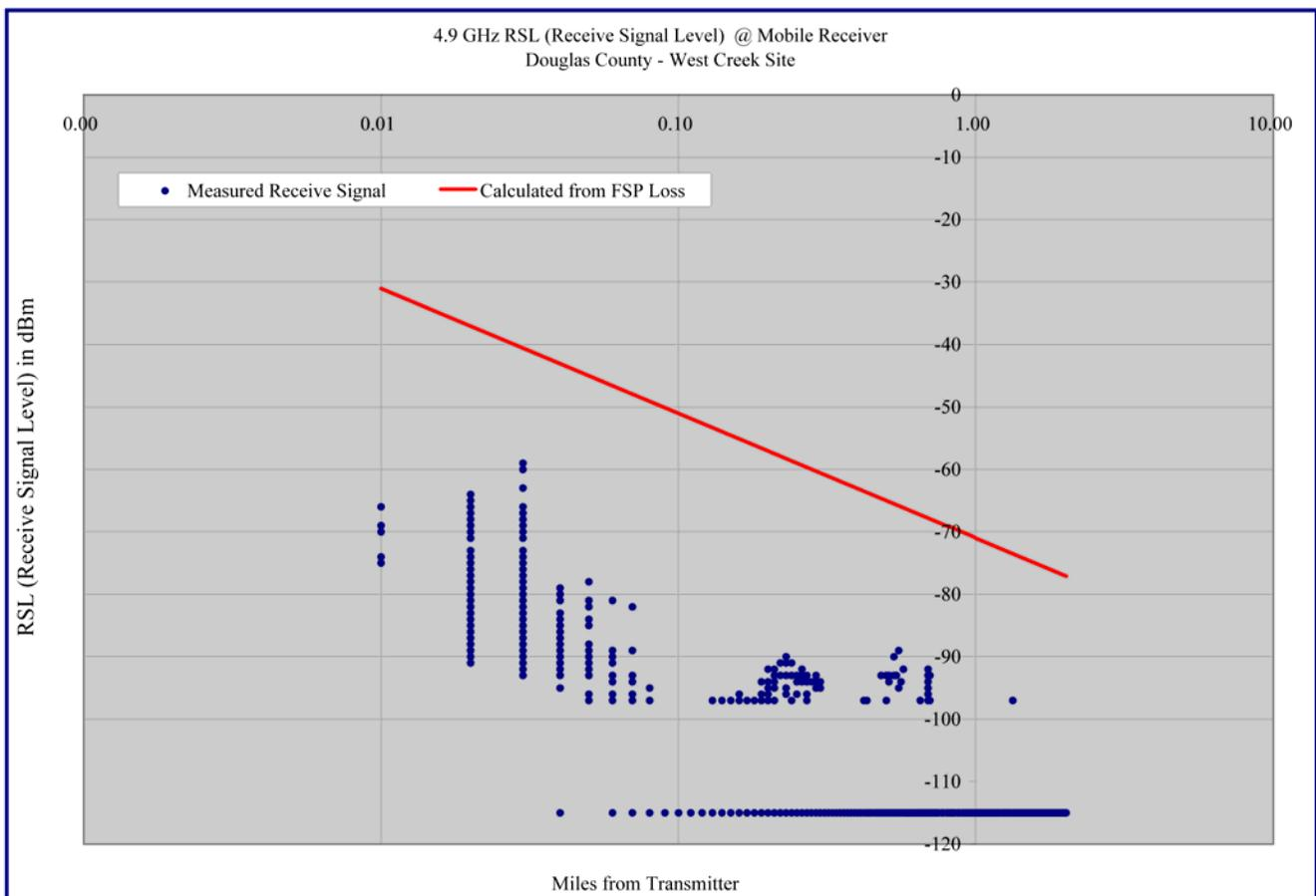
**Graph 3.6 - West Creek –Predicted Receive Signal Level versus Distance – Log-Log Format**
