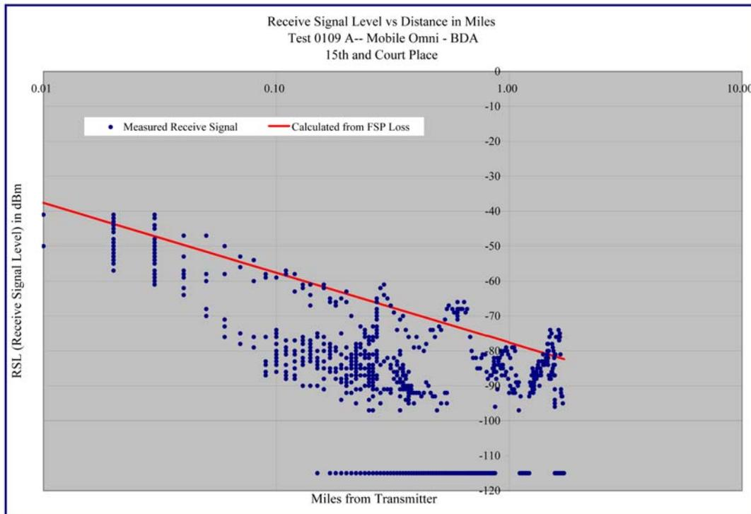
Graph 6.34 – Receive Signal Level versus Distance – 15<sup>th</sup> and Court Place – Log-Log Format
