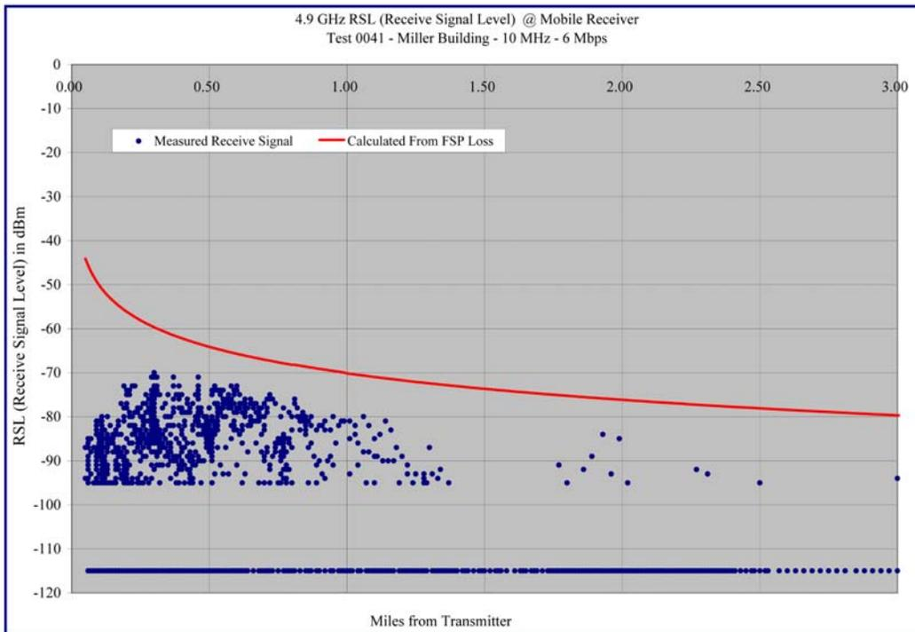
**Graph 4.10 – Miller Building – 10 MHz/ 6 Mbps - Receive Signal versus Distance**
