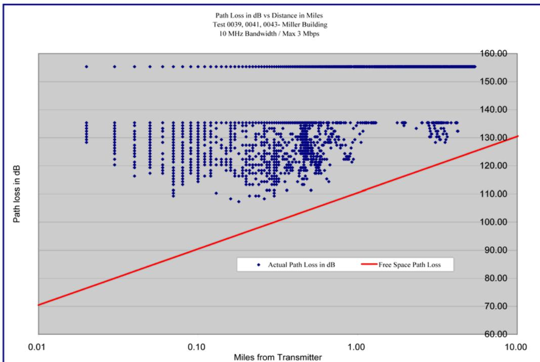
**Graph 4.8 – Miller Building – 10 MHz / 3 Mbps – Path Loss versus Distance in Miles – Log-Log Format**
