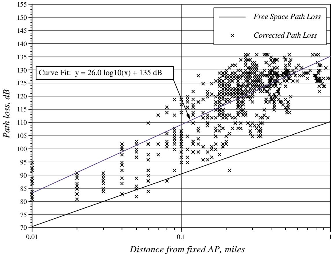
Figure 11- Path Loss Versus Distance for Test 105
