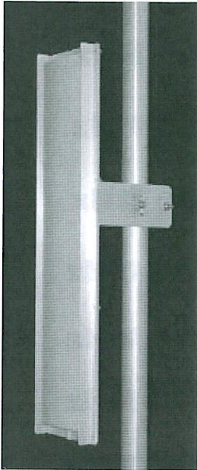
The TA-4904-14-90 is a vertically polarized 90 degree sectoral antenna. The antenna consists of a printed dipole array enclosed in an aluminum base with a UV stabilized radome for superior weatherability. The antenna is at DC ground to aid in lightning protection.
