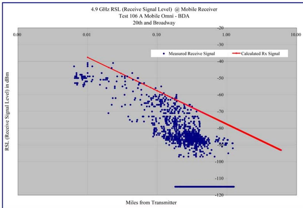
**Graph 6.10 – Receive Signal versus Distance – 20<sup>th</sup> and Broadway – Log-Log Format**
