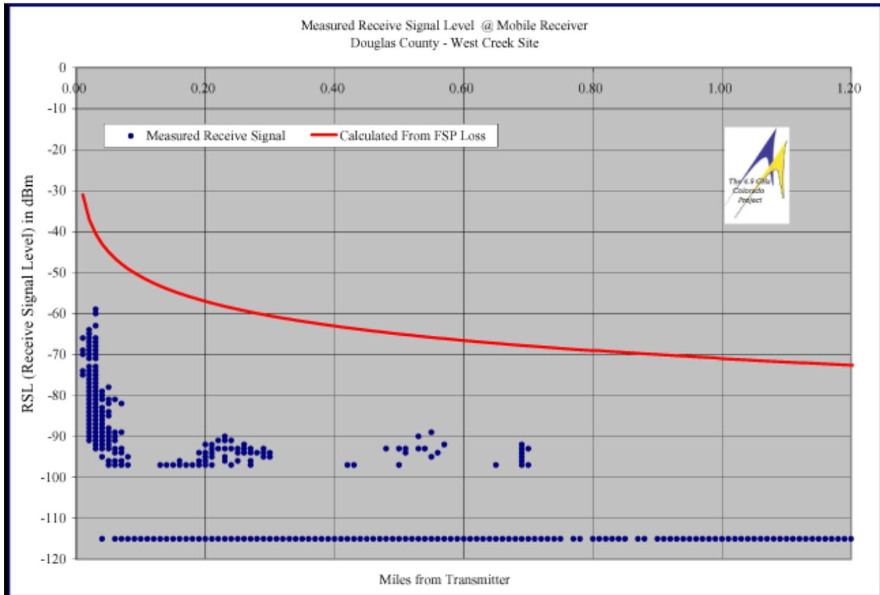
**Graph 3.5 - West Creek - Predicted Receive Signal Level versus Distance**
