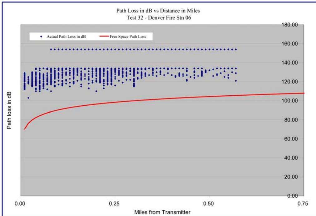
**Graph 5.3 – Denver Fire Station 06 - Path Loss versus Distance**
