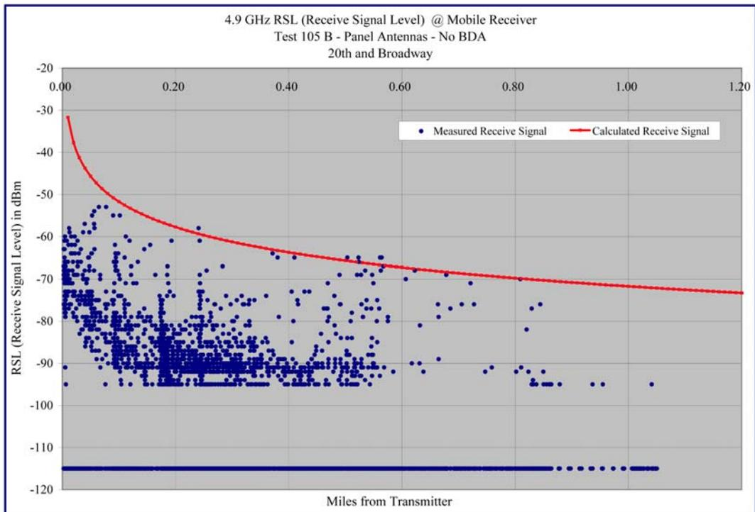
**Graph 6.5 – Receive Signal Level versus Distance – Test 105B – Panel Antennas no BDA**
