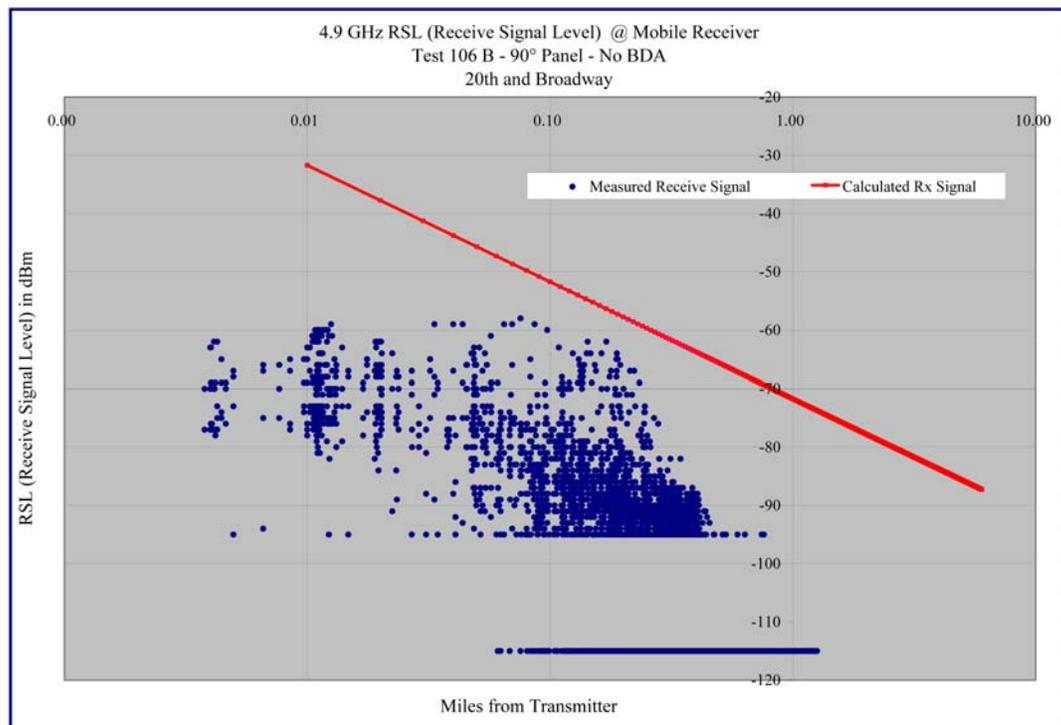
**Graph 6.14 – Receive Signal Level versus Distance – 20<sup>th</sup> and Broadway Test B – Log-Log Format**
