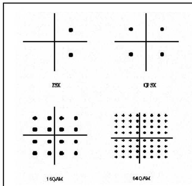
Figure 2.2– Schematic of Modulation Types
