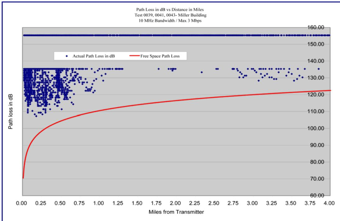
**Graph 4.6 – Miller Building – 10 MHz / 3 Mbps – Path Loss versus Distance in Miles**
