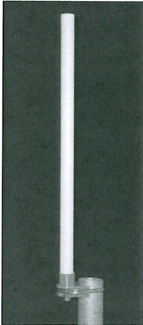
The TA-4952 is a 10 dBi omnidirectional antenna consisting of end fed collinear dipoles in a UV stabilized fiberglass radome. The antenna is designed for severe weather conditions and is at DC ground to aid in lightning protection. The TA-4952 has been developed in response to customer requests specifically with and for the Public Safety Band in mind which demands optimal performance and reliability at an affordable price.
