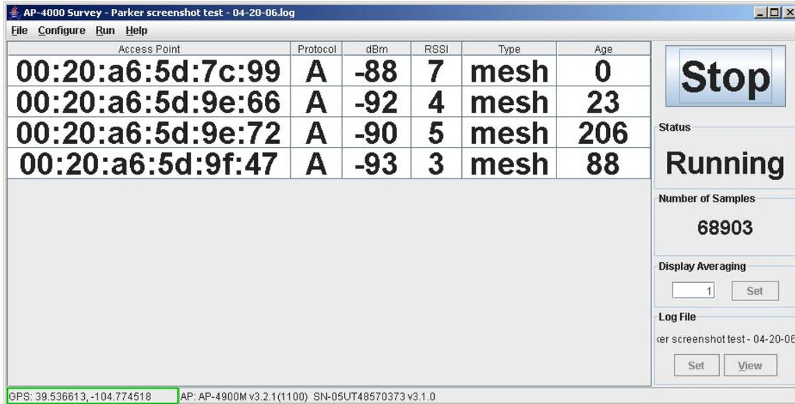
Figure 7 - Screen Shot of Survey Software Window
