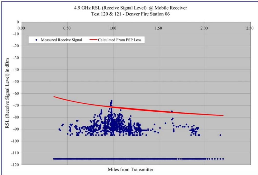
**Graph 5.5 – Receive Signal Level versus Distance - Denver Fire Station 06**
