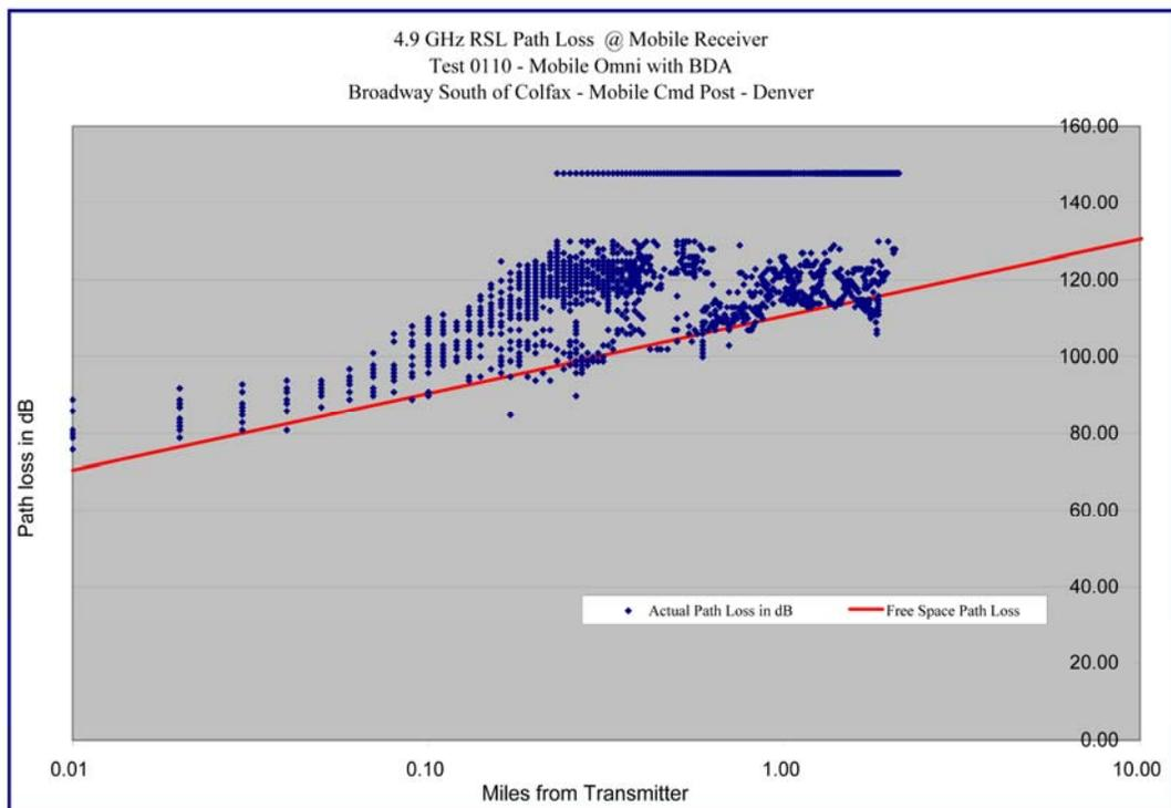
**Graph 6.44 Path Loss versus Distance – Broadway South of Colfax – Log-Log Format**
