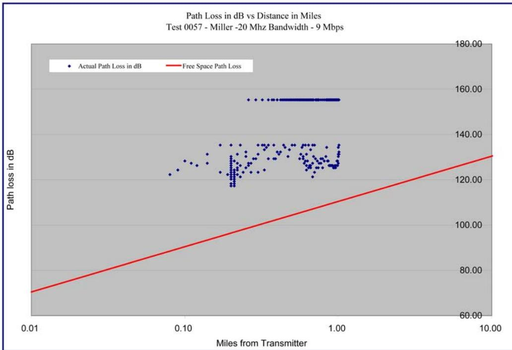
**Graph 4.32 – Miller Building - 20 MHz / 9 Mbps – Path Loss versus Distance – Log-Log Format**
