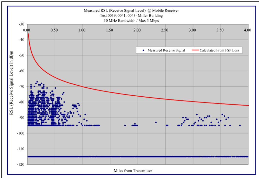
**Graph 4.2 – Miller Building – 10 MHz / 3 Mbps - Receive Signal Level versus Distance**
