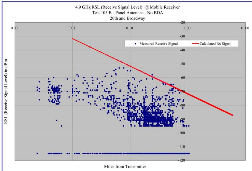
**Graph 6.6 – Receive Signal Level versus Distance – Test 105B – Panel Antennas no BDA – Log-Log Format**
