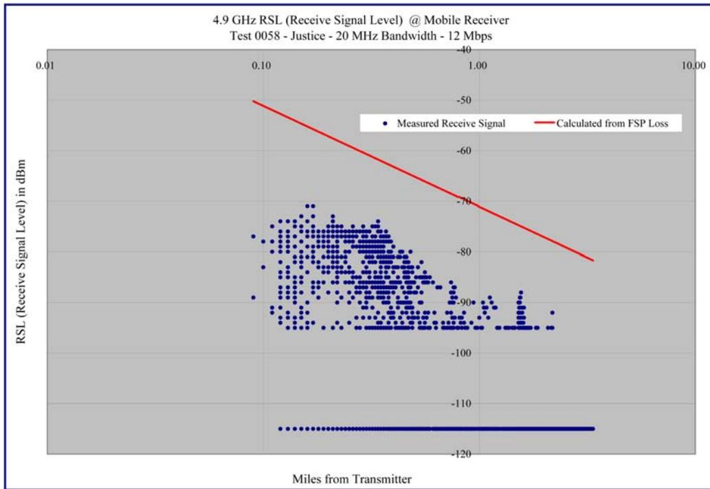
**Graph 4.35 – Justice Center - 20 MHz / 12 Mbps - Receive Signal Strength versus Distance- Log-Log Format**
