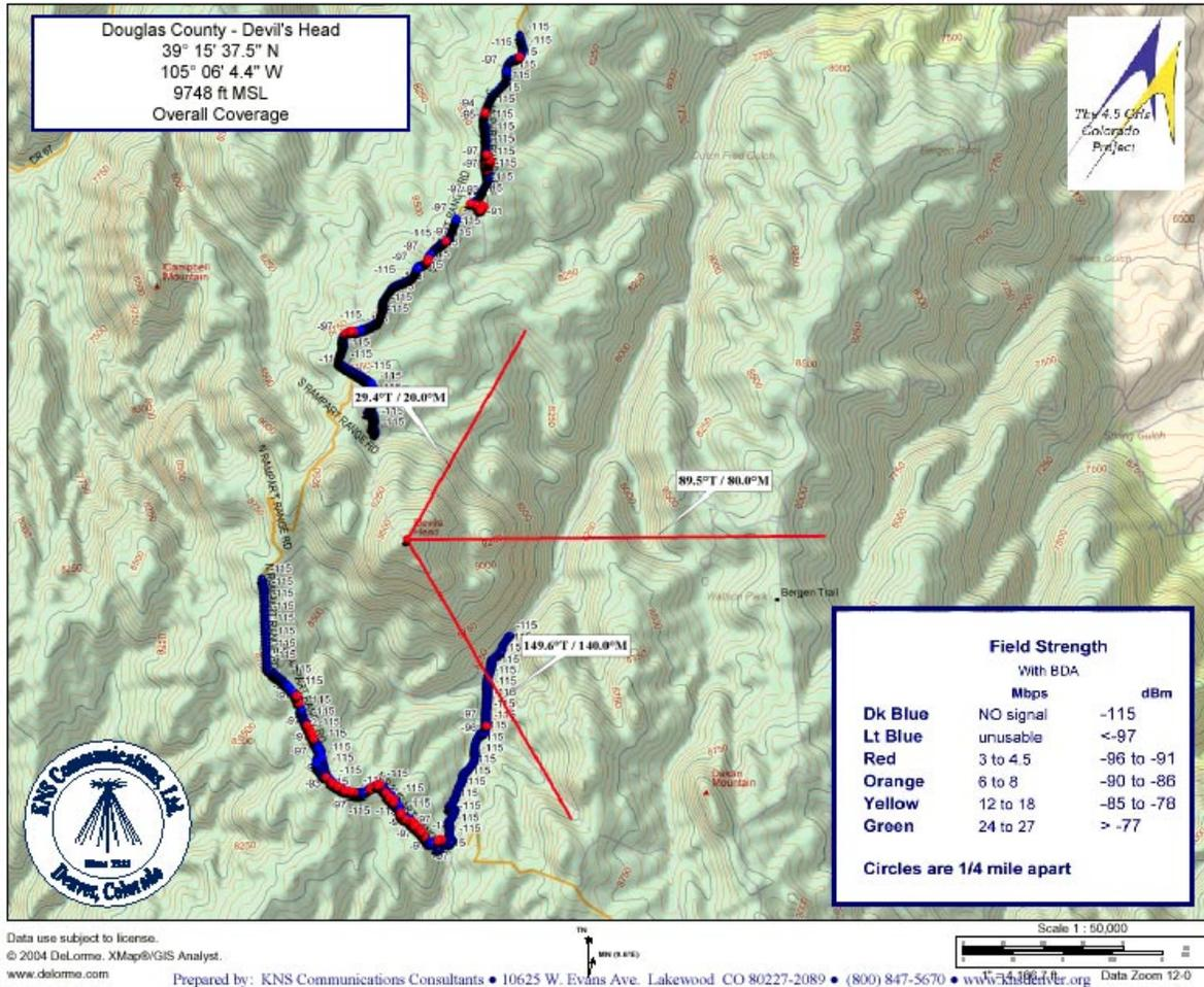
Figure 16 - Devil's Head Coverage (EIRP = 31 dBm)
