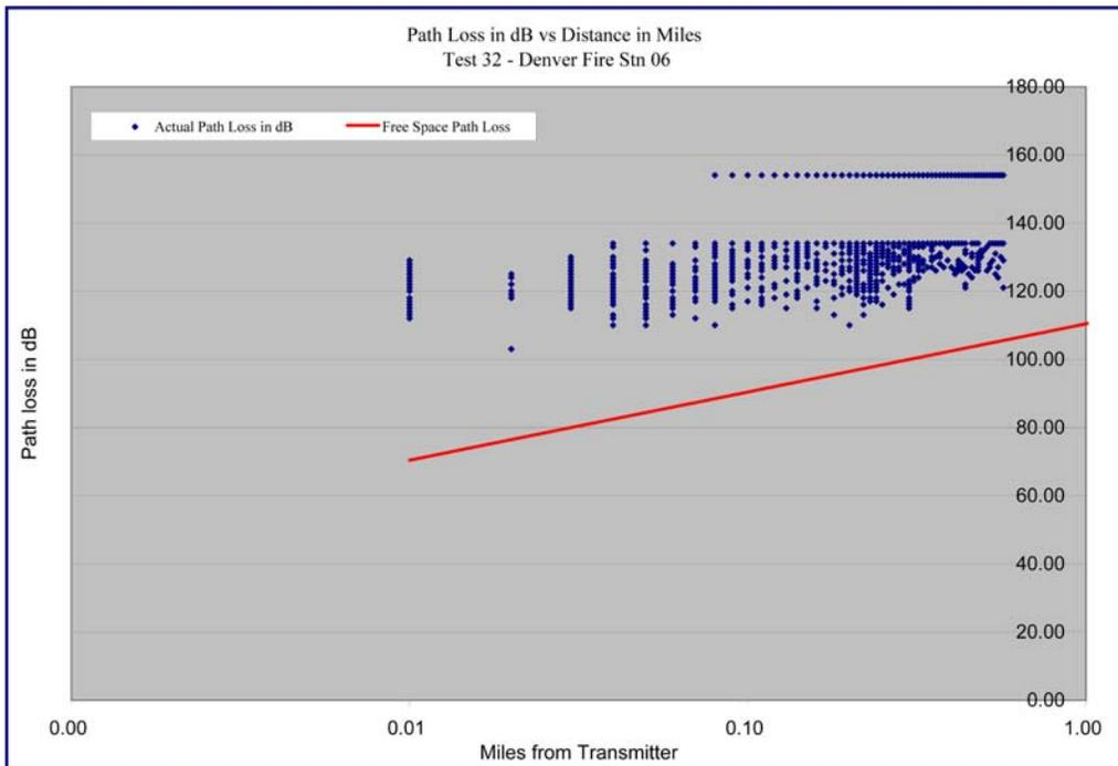
**Graph 5.4 -- Station Fire Station 06 - Path Loss versus Distance-- Log-Log Format**
