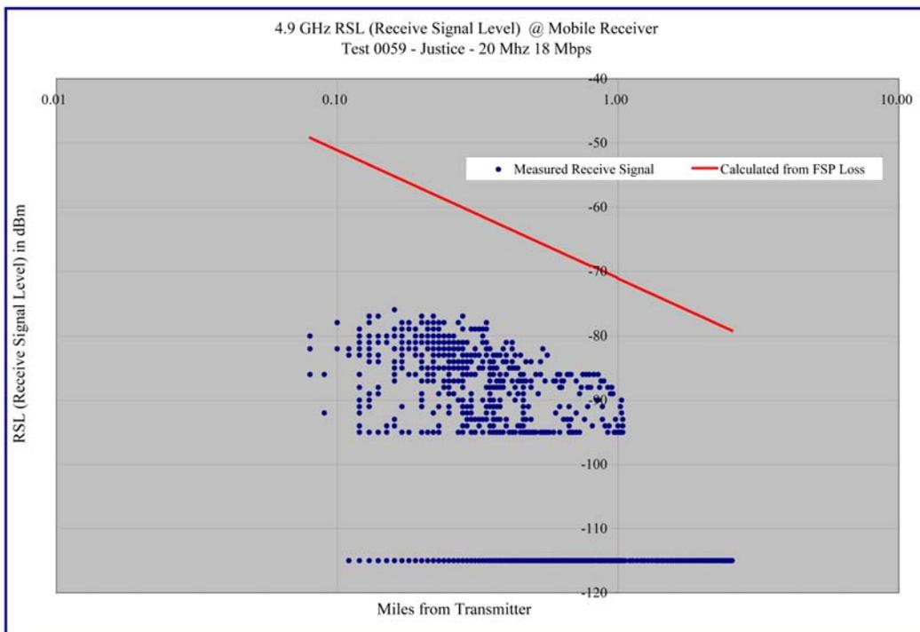
**Graph 4.50 – Justice Center -- 20 MHz / 18 Mbps - Receive Signal Strength versus Distance – Log-Log Format**
