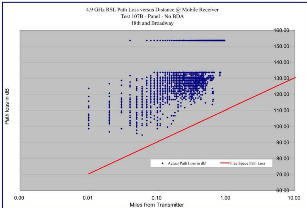
**Graph 6.24 – Path Loss versus Distance – Test 107B – 18<sup>th</sup> and Broadway – Log-Log Format**
