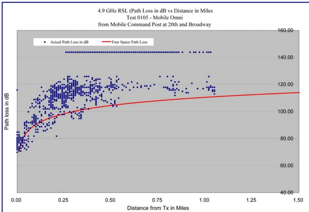
**Graph 6.3 – Path Loss versus Distance – Test 105 Omni with BDA**
