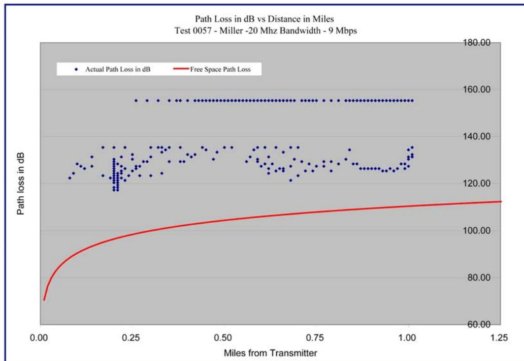
Graph 4.30 – Miller Building- 20 MHz / 9 Mbps – Path Loss versus Distance
