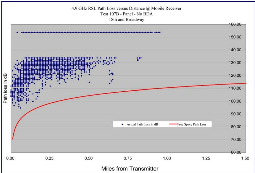
**Graph 6.23 – Path Loss versus Distance – Test 107B – 18<sup>th</sup> and Broadway**
