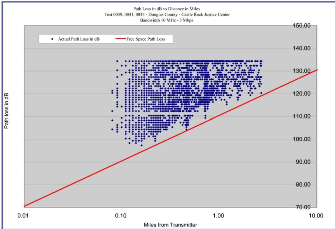
**Graph 4.7 – Justice Center – 10 MHz / 3 Mbps - Path Loss versus Distance in Miles – Log-Log Format**
