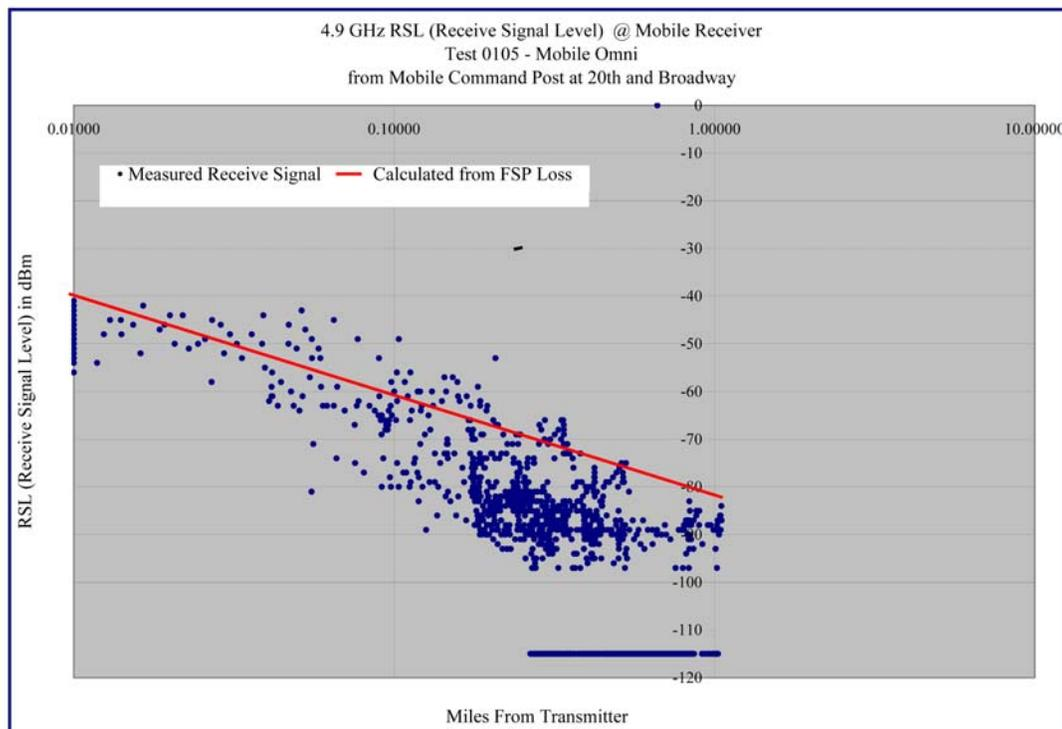
**Graph 6.2 – Receive Signal Level versus Distance – Test 105 Omni with BDA – Log-Log Format**
