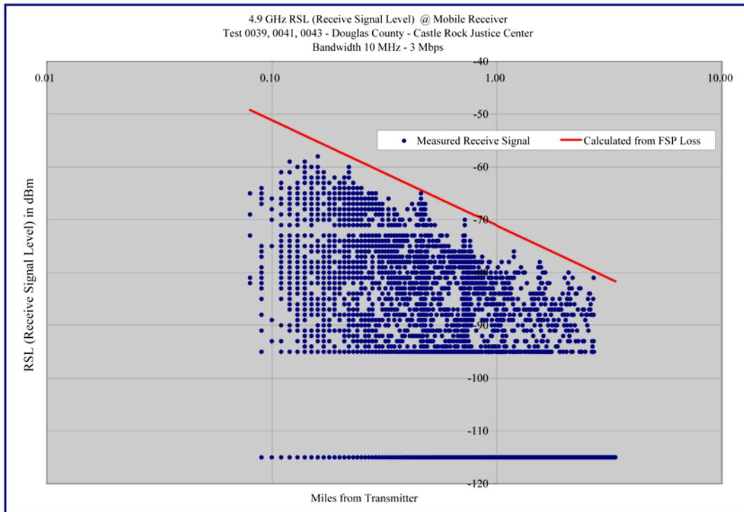
**Graph 4.3 – Justice Center – 10 MHz / 3 Mbps - Receive Signal Level Versus Distance-Log-Log**
