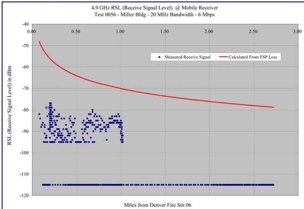
**Graph 4.18 – Miller Building – 20 MHz / 6 Mbps - Receive Signal versus Distance**
