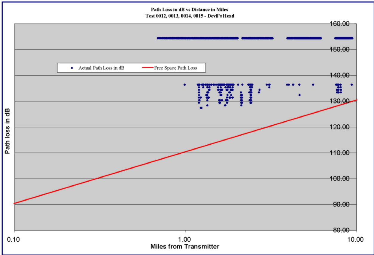
**Graph 3.4 - Measured Path Loss versus Distance – Log-Log format – Devil’s Head**
