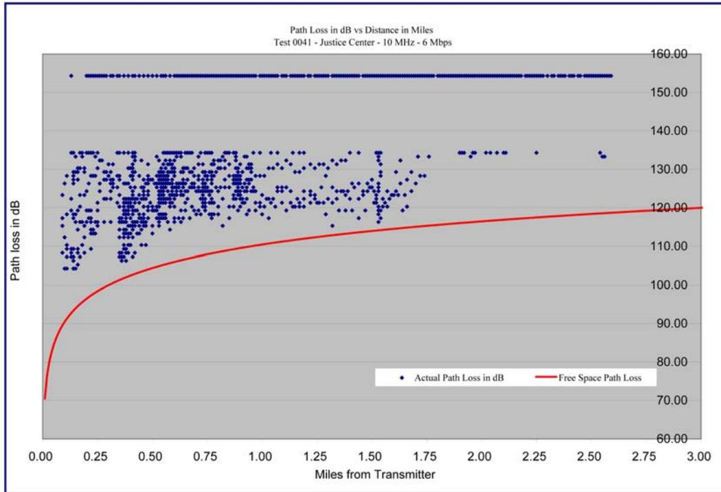
**Graph 4.13– Justice Center – 10 MHz / 6 Mbps– Path Loss versus Distance**
