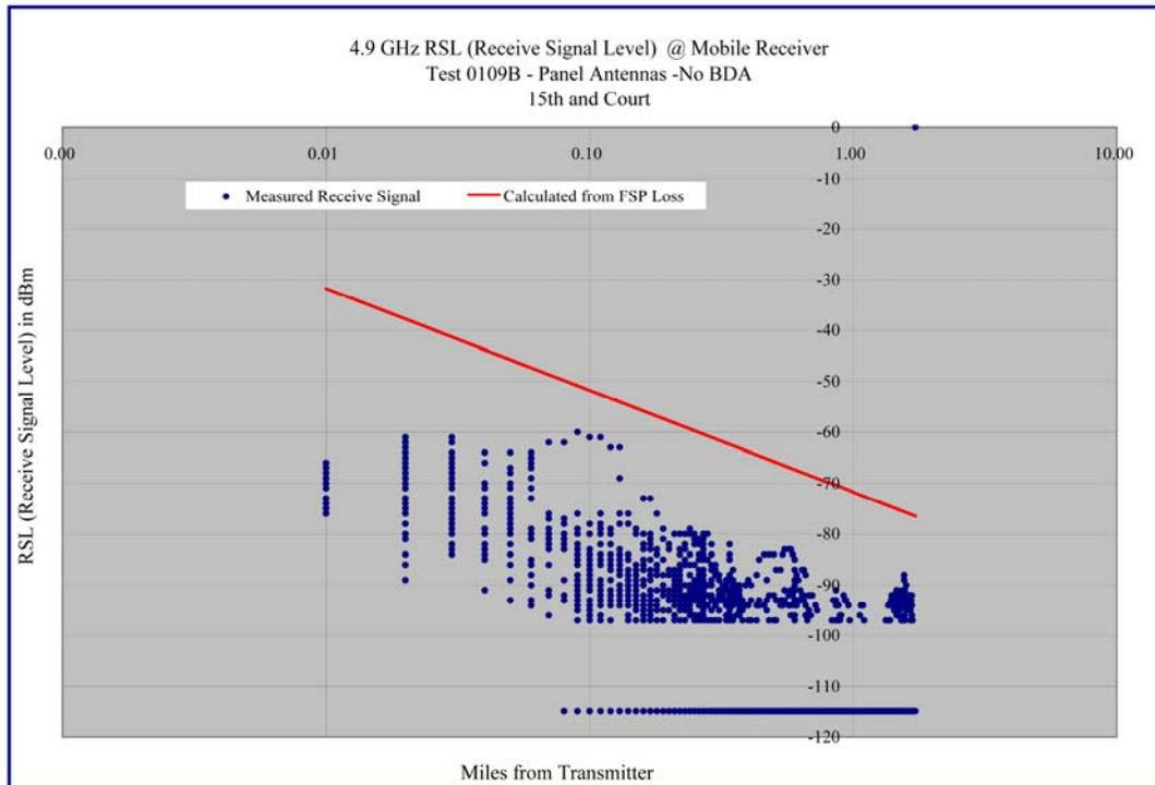
Graph 6.38 Receive Signal Level versus Distance – 15<sup>th</sup> and Court Place – Log-Log Format
