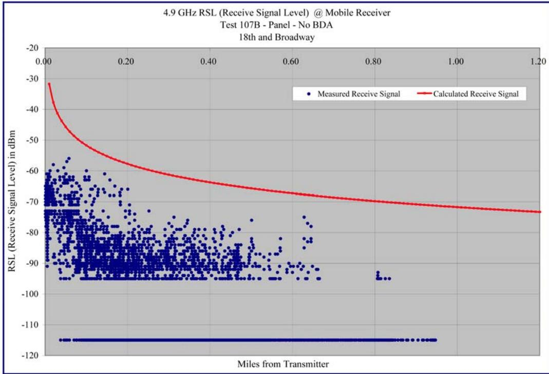
Graph 6.21 – Receive Signal Level versus Distance – Test 107B – 18<sup>th</sup> and Broadway
