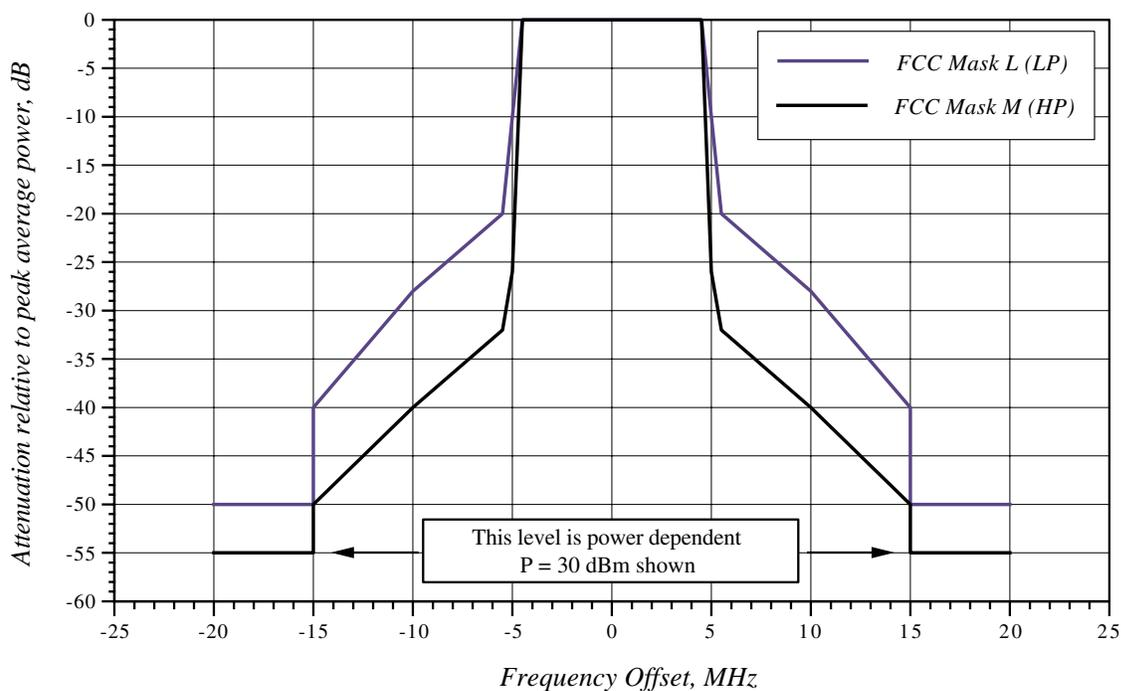
Figure 1 - FCC 10 MHz Emission Masks
