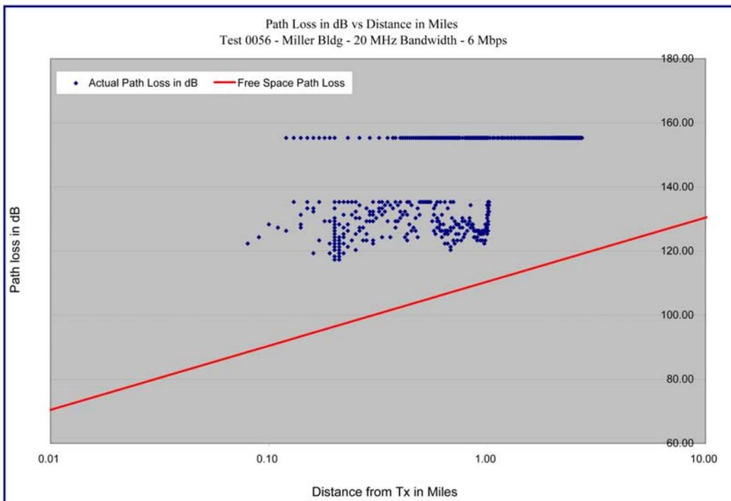
Graph 4.24 – Miller Building – Path Loss versus Distance – 20 MHz / 6 Mbps – Log-Log Format
