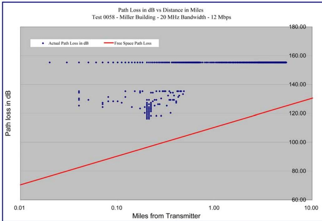
**Graph 4.40 – Miller Building - 20 MHz / 12 Mbps - Path Loss versus Distance – Log-Log Format**
