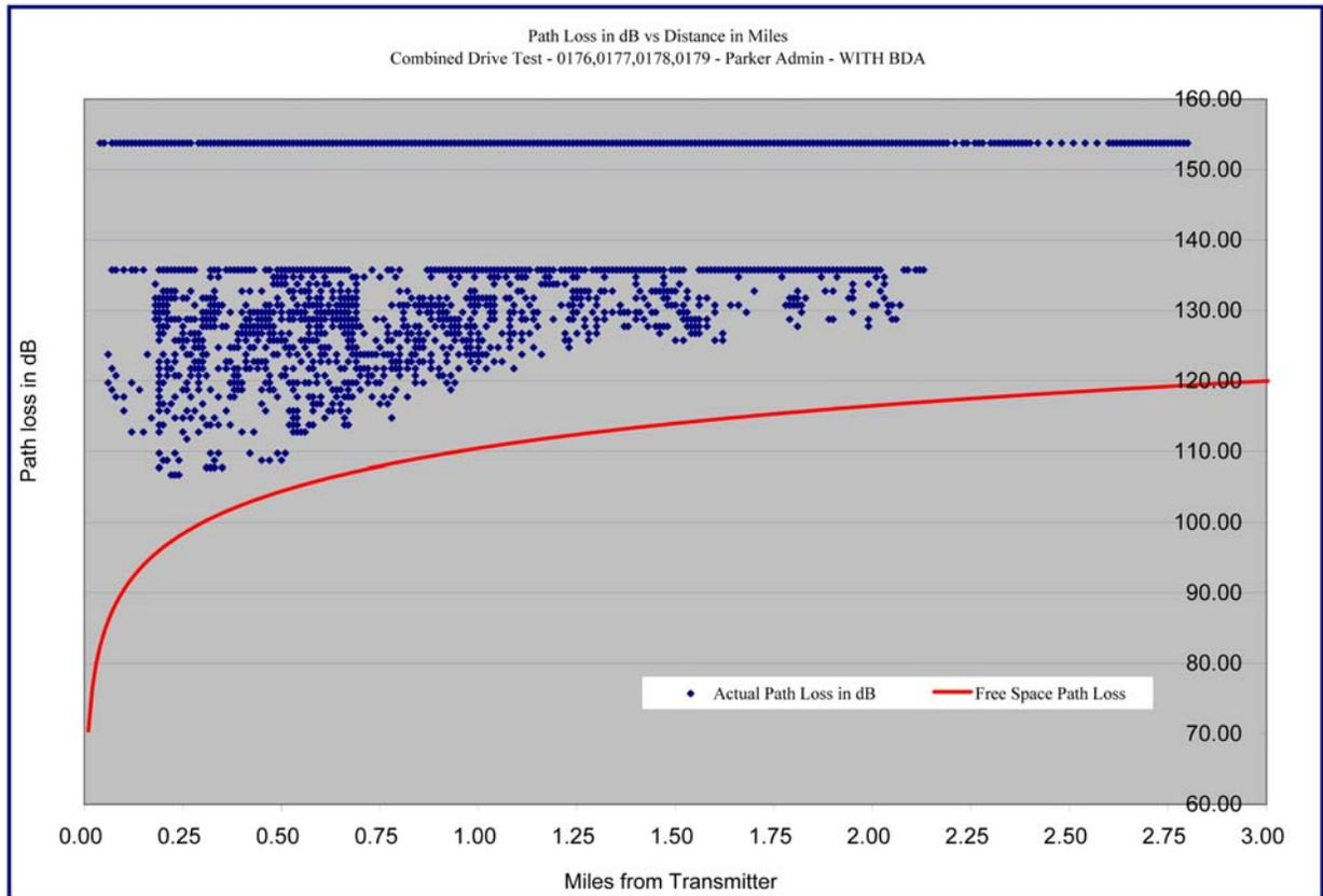
**Graph 2.3 - Measured Free Space Path Loss versus Distance**
