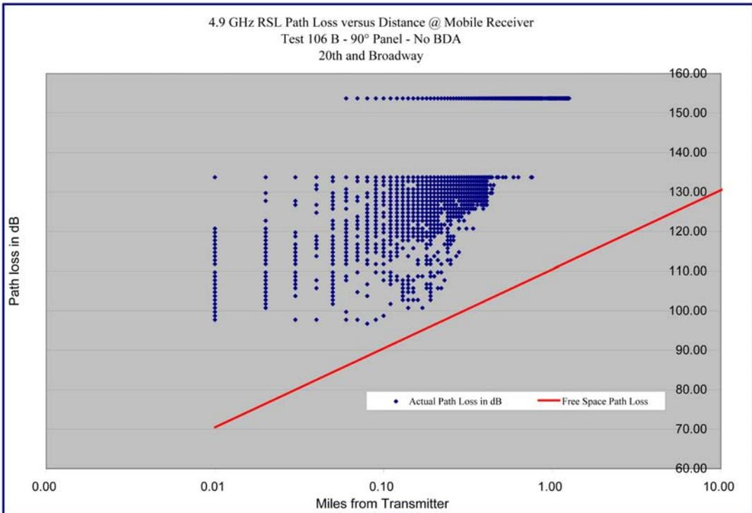
**Graph 6.16 – Path Loss versus Distance – 20<sup>th</sup> and Broadway Test B – Log-Log Format**
