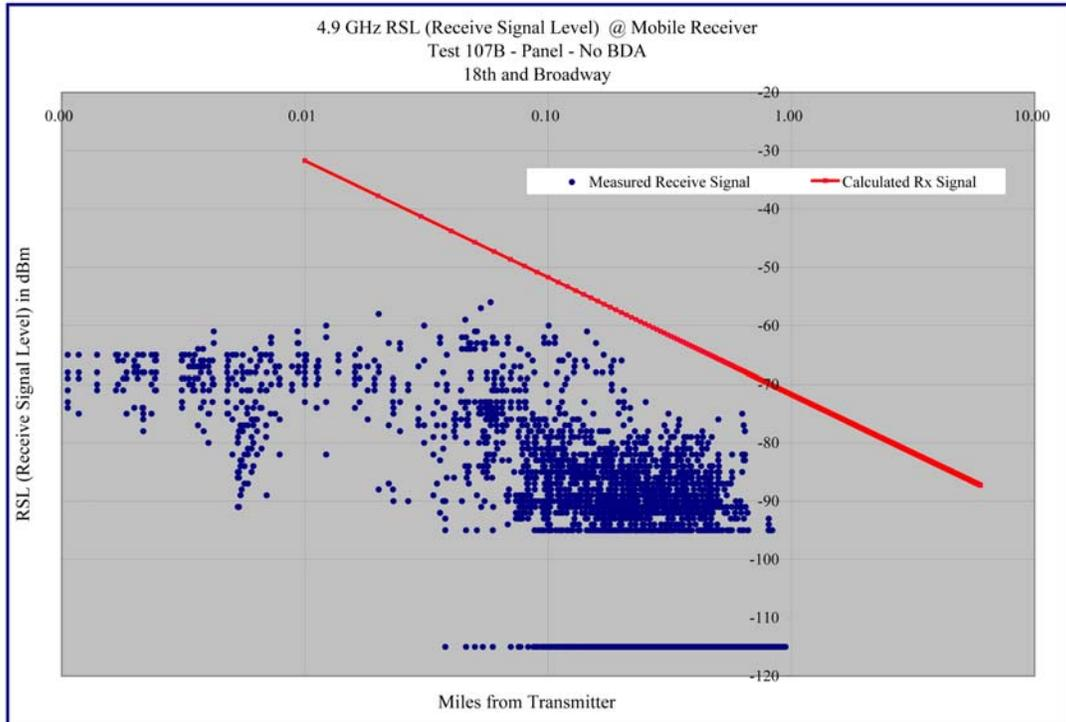
Graph 6.22 – Receive Signal Level versus Distance – Test 107B – 18<sup>th</sup> and Broadway – Log-Log Format
