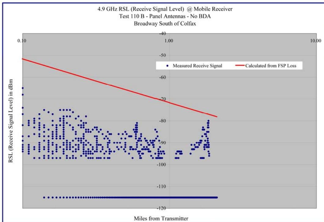
Graph 6.46 Receive Signal Level versus Distance – Broadway South of Colfax – Log-Log Format
