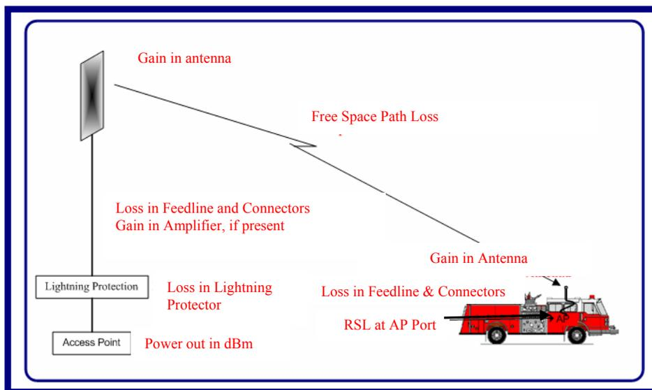
**Figure 2.1 - Calculation of Theoretical Receive Signal Level In Mobile**
