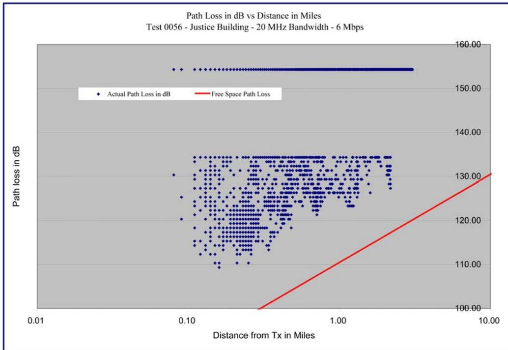
Graph 4.23 – Justice Center – Path Loss versus Distance – 20 MHz / 6 Mbps – Log-Log Format
