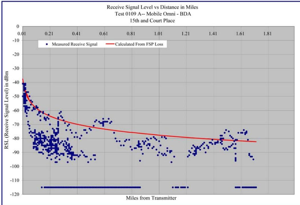
Graph 6.33 – Receive Signal Level versus Distance – 15<sup>th</sup> and Court Place
