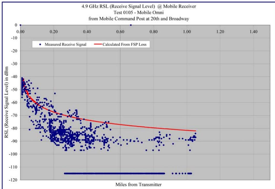
**Graph 6.1 – Receive Signal Level versus Distance – Test 105 Omni with BDA**
