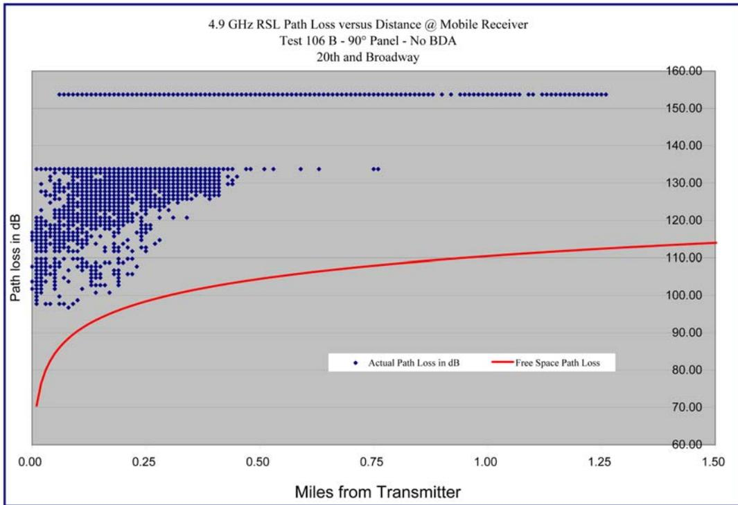
**Graph 6.15 – Path Loss versus Distance – 20<sup>th</sup> and Broadway Test B**
