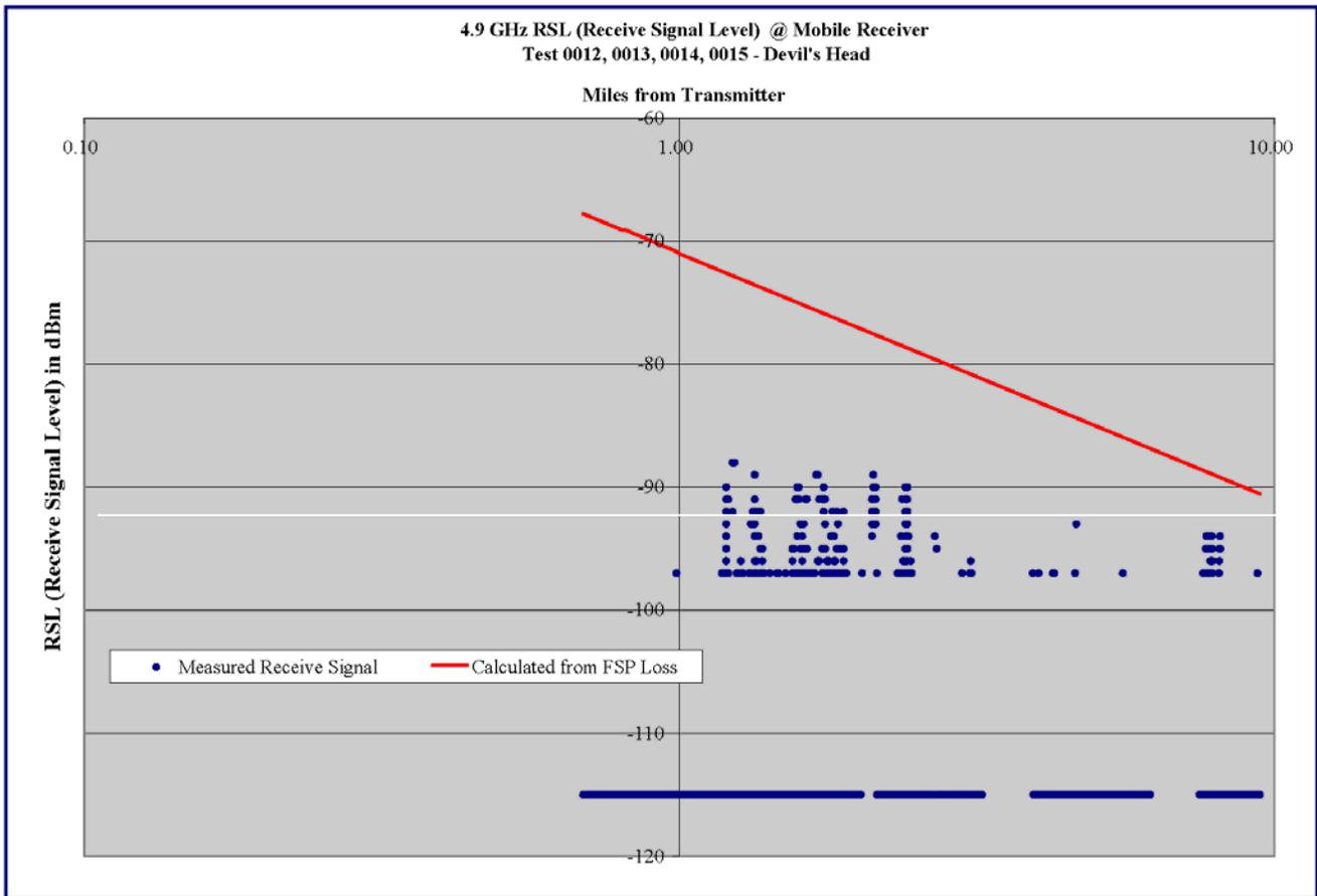
**Graph 3.2 - Measured Receive Signal versus Distance – Log-Log Format – Devil’s Head**
