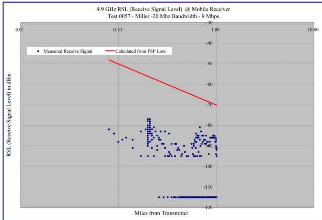
**Graph 4.28 – Miller Building - 20 MHz / 9 Mbps – Receive Signal Strength versus Distance – Log-Log Format**
