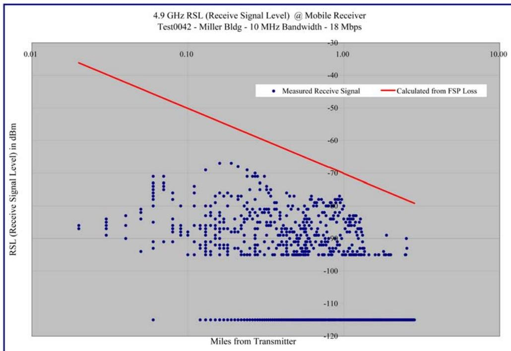
**Graph 4.44 – Miller Building -10 MHz / 18 Mbps - Receive Signal Strength versus Distance- Log-Log Format**
