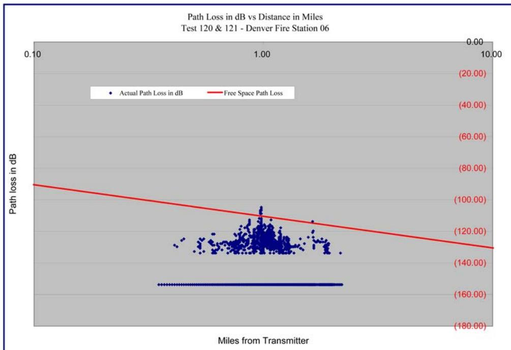
**Graph 5.8 – Path Loss versus Distance – Log-Log Format – Denver Fire Station 06**
