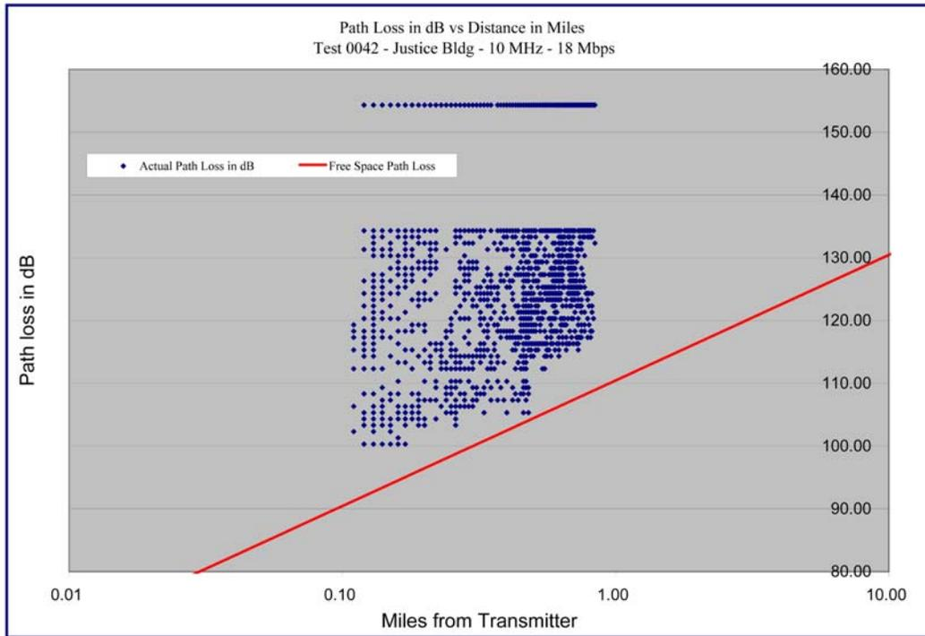
**Graph 4.47 – Justice Center - 10 MHz / 18 Mbps - Path Loss versus Distance – Log-Log Format**
