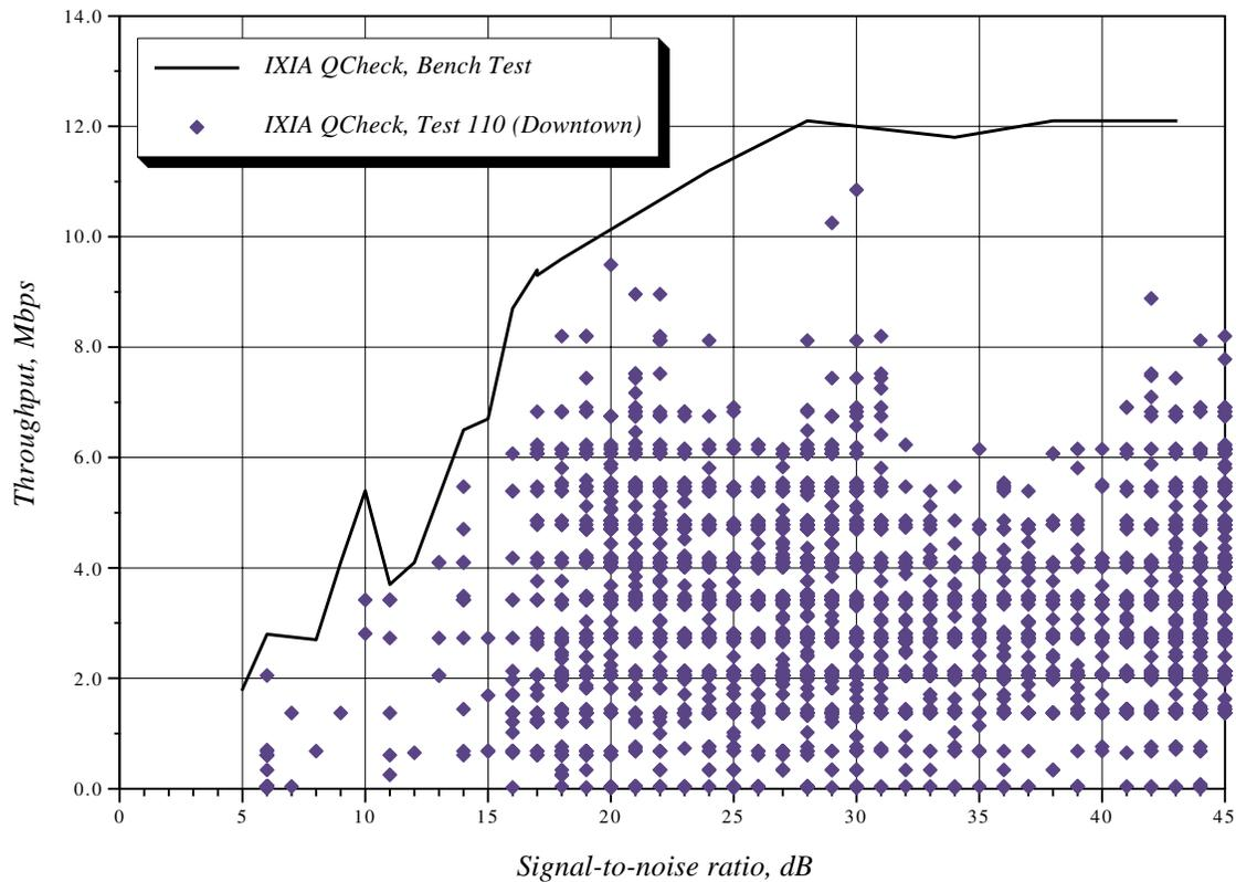
Figure 13 - Transport Layer Throughput, AP-4900, 10 MHz Channel
