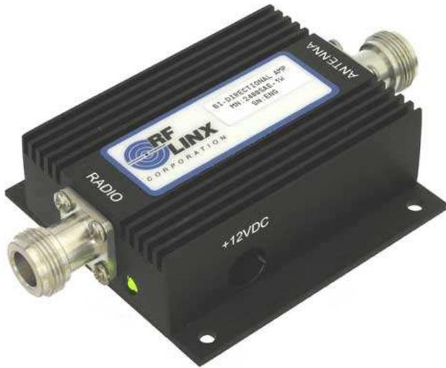
The Antennafier™ 4900-5800 S series Bi-Directional Amplifiers will significantly improve link reliability and operating range by providing Low Noise Amplification during Receive, and Spectrally Clean Power Amplification during Transmit. These fixed gain devices housed in a rugged machined aluminum chassis and are available in either indoor or outdoor models covering 4.9 to 5.8GHz in five popular bands.
