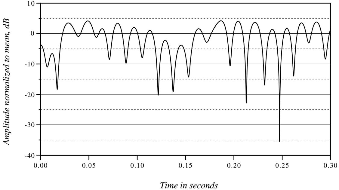
Figure 2 - Time-Varying Amplitude on Rayleigh Fading Channel
