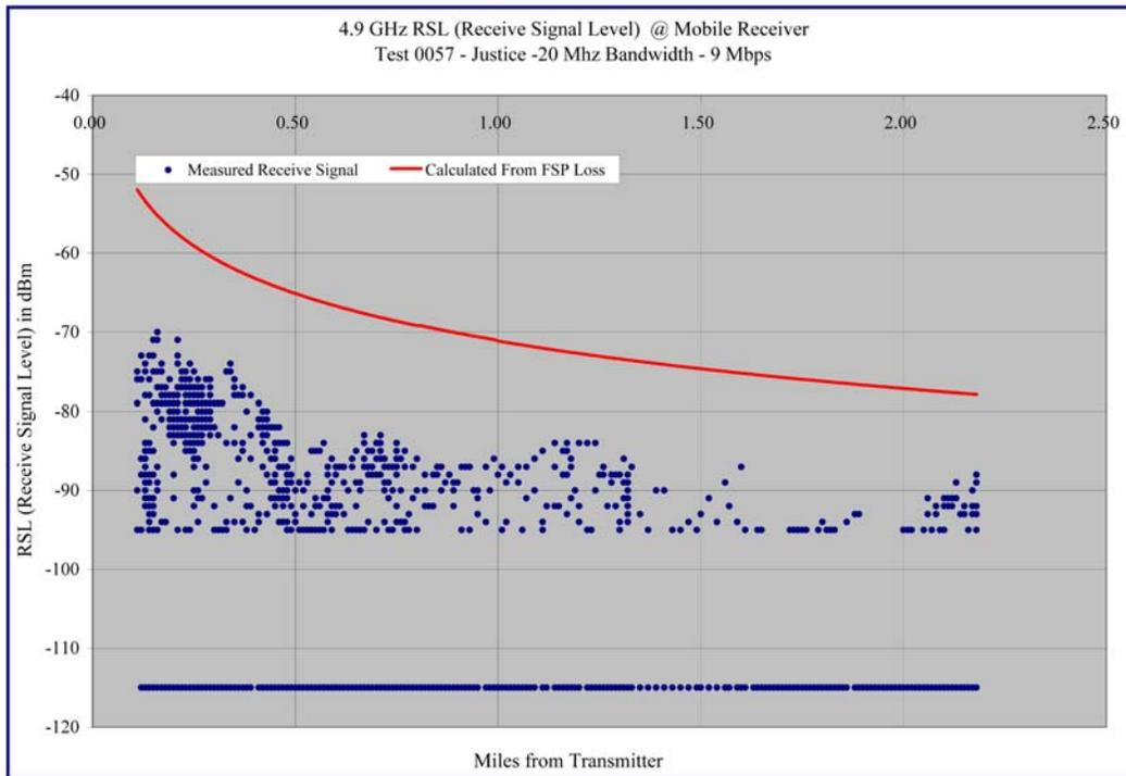
**Graph 4.25 – Justice Center – 20 MHz / 9 Mbps - Receive Signal Strength versus Distance**
