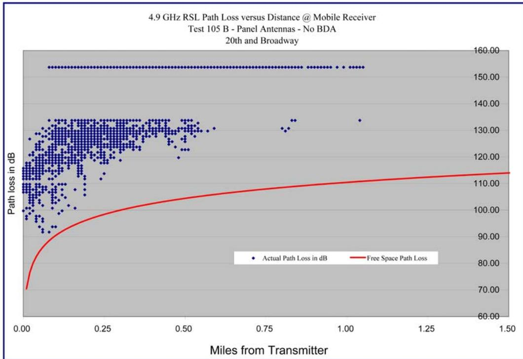
**Graph 6.7 – Path Loss versus Distance – Test 105B – Panel Antennas no BDA**
