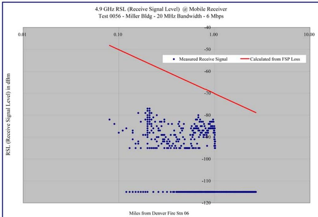
Graph 4.20 Miller Building – Receive Signal Level versus Distance – 20 MHz / 6 Mbps – Log-Log Format
